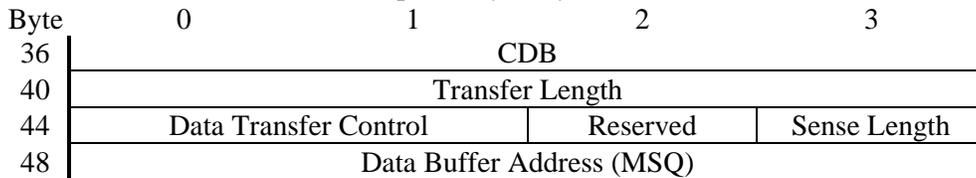
The Data Transfer Control doublet will be structured as four 4-bit fields:
