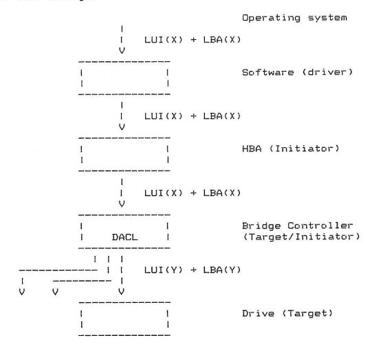
7.5 Branch with Multiple Layers of SCSI Disk Arrays
