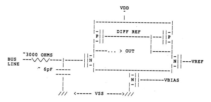
The "..." prior to the electrically accessible output indicates other digital circuitry that will produce delay but not bit errors
