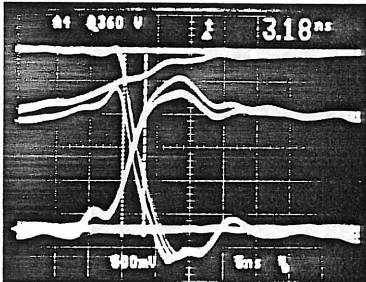
ABOVE REFLECTION AND CROSSTALK IN PERIPHERAL Ø, LINE 3 OUTPUT:
