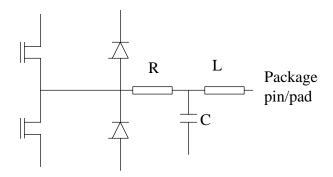
Output is the values of the R, L, C components, the IV curves for the transistors and diodes, simple rise and fall times
