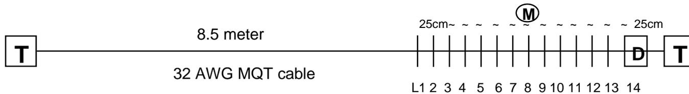
“setup & hold time measurements for 12 m 32 AWG MQT cable”
