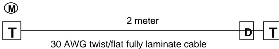
“setup & hold time measurements for 2 m 30 AWG cable”
