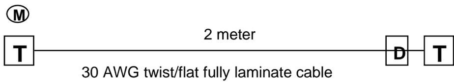
“setup & hold time measurements for 2 m 30 AWG cable”
