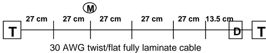
“setup & hold time measurements for 1.5 m 30 AWG cable”
