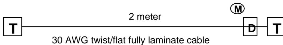
“setup & hold time measurements for 2 m 30 AWG cable”
