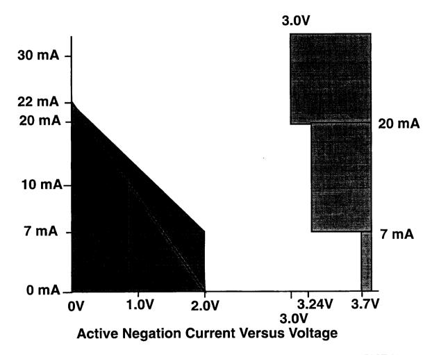
The figure white area is the current range of an active negation driver as defined in FAST-20. This specifies both the minimum and maximum currents allowed over the active negation voltage range. Once the voltage is over 3,24 Volts, the driver must not source more than 7 mA.
