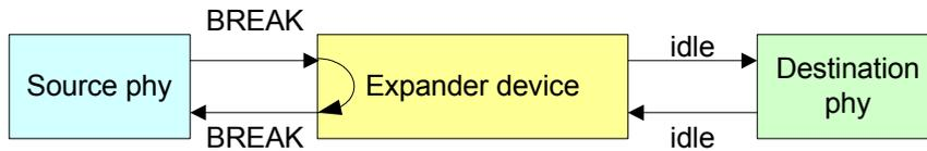
Case 2: OPEN address frame has propagated through the expander device:
