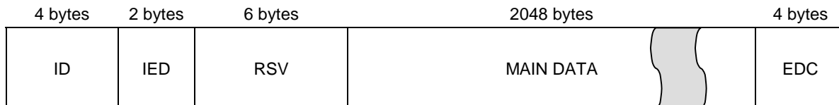
Figure 2 – Logical Layout of a DVD+RW Data Sector
