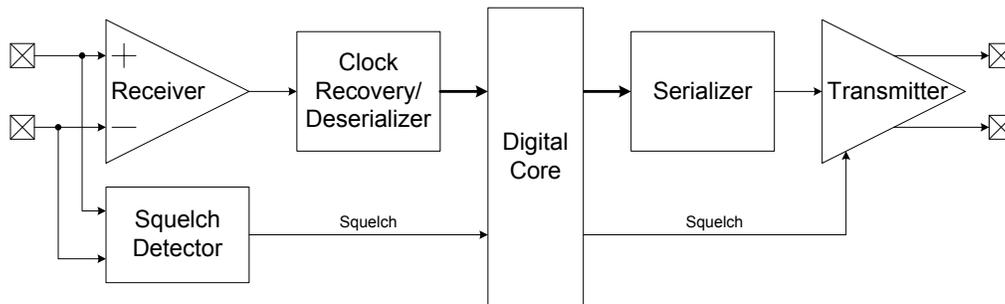
Bandwidth requirements for the signal path are well known from other protocols; in order to pass data through the signal path (including the channel, connectors, package, and any buffering) a minimum raw bandwidth of about 70% of the bit rate is required. In other words, a 3,0 Gbps system requires a signal path bandwidth of 2,1 GHz or higher.
