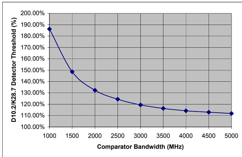
As can be seen, in order to minimize the frequency-dependent effects, the comparator bandwidth must be maximized, and in fact even with a bandwidth of 4,5 GHz there is still an amplitude error of 13%. In practice, additional second order effects (not modeled in these simulations) tend to accumulate, increasing the frequency-dependent amplitude error even more.
