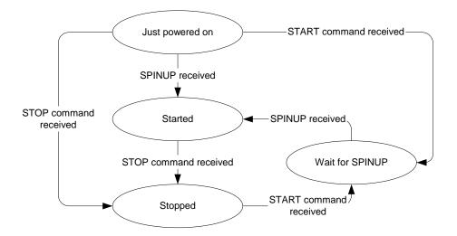
The enclosure shall generate SPINUP after power on whenever it wants to allow the disk drive to spin-up. It may choose to rotate SPINUP across all its ports (distributing it to N ports at a time if the enclosure power supply is capable of powering up N drives at a time).
