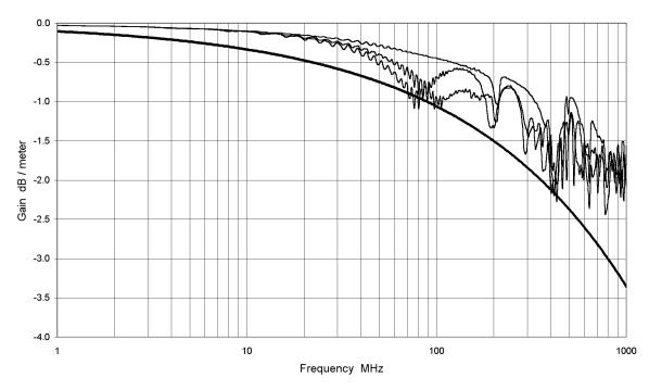
Figure 4 - Attenuation of 3 different pairs, mask added
