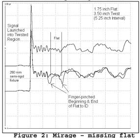
Figure 2 shows that we may not be able to trust  $\ensuremath{\mathtt{TDR}}$  readings for flats measured near the fixture.
