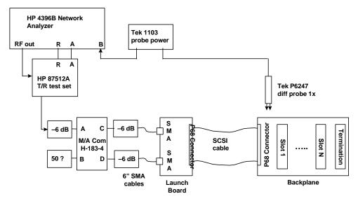
For cable-only measurements active terminator or resistive loads were used in place of backplane
