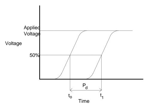
Figure 3 - Propagation time measurements
