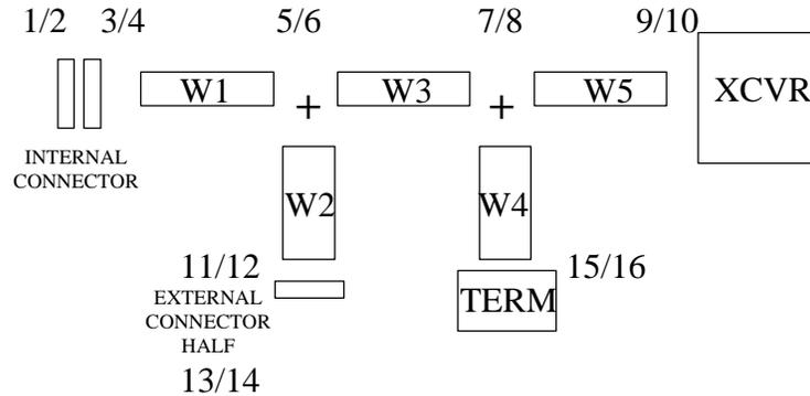
Figure 2 - Architecture of a transceiver board model (no unused connectors)
