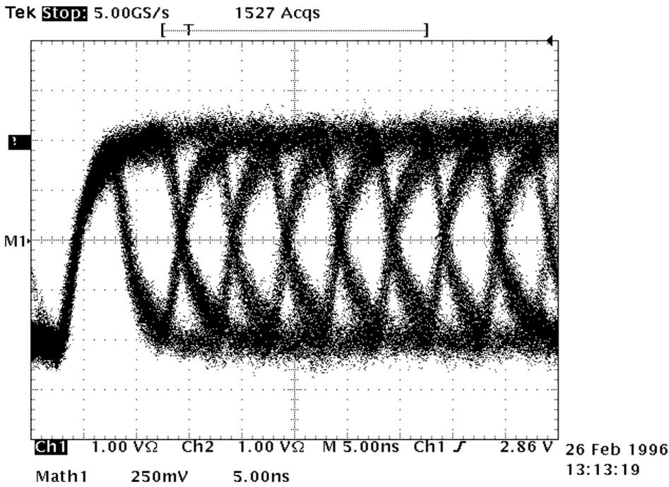
Figure 22: SSA RX Eye Diagram: 20MB/s, 30.0 meter cable
