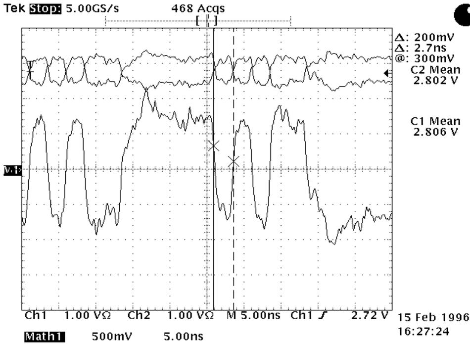
Figure 11: SSA Waveform: 40MB/s, single trigger, 0.6 meter cable
