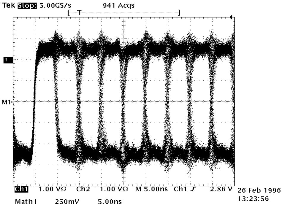
Figure 20: SSA RX Eye Diagram: 20MB/s, 2.0 meter cable
