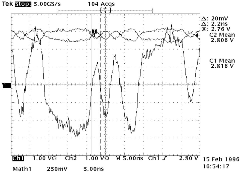
Figure 13: SSA Waveform: 40MB/s, single trigger, 20.0 meter cable
