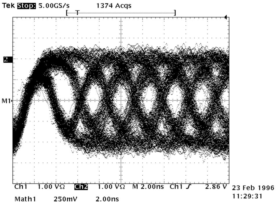
Figure 26: SSA RX Eye Diagram: 40MB/s, 20.0 meter cable
