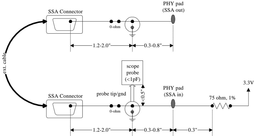
Figure 3: SSA Signal Routing/Probing
