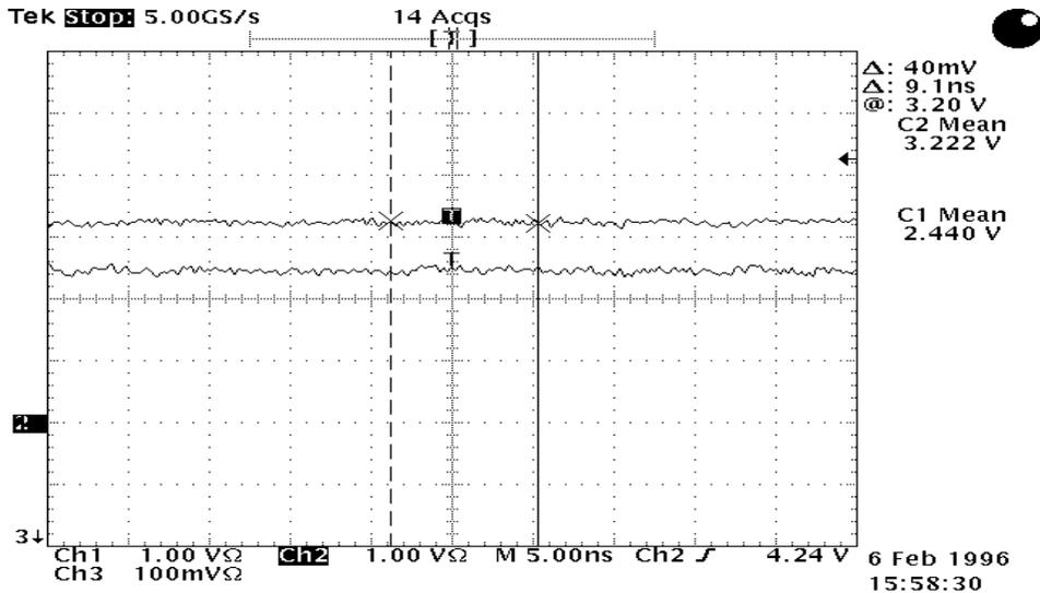
Figure 9: SSA Waveform: Link driver in wrap mode
