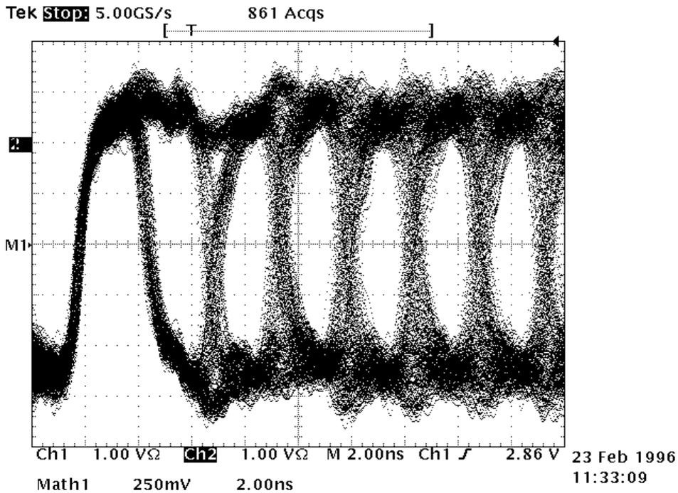
Figure 23: SSA RX Eye Diagram: 40MB/s, 0.3 meter cable
