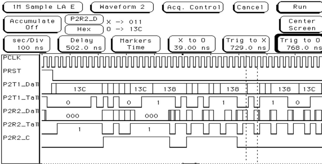
Figure 5: Protocol Waveform: 20MB/s normal mode from reset
