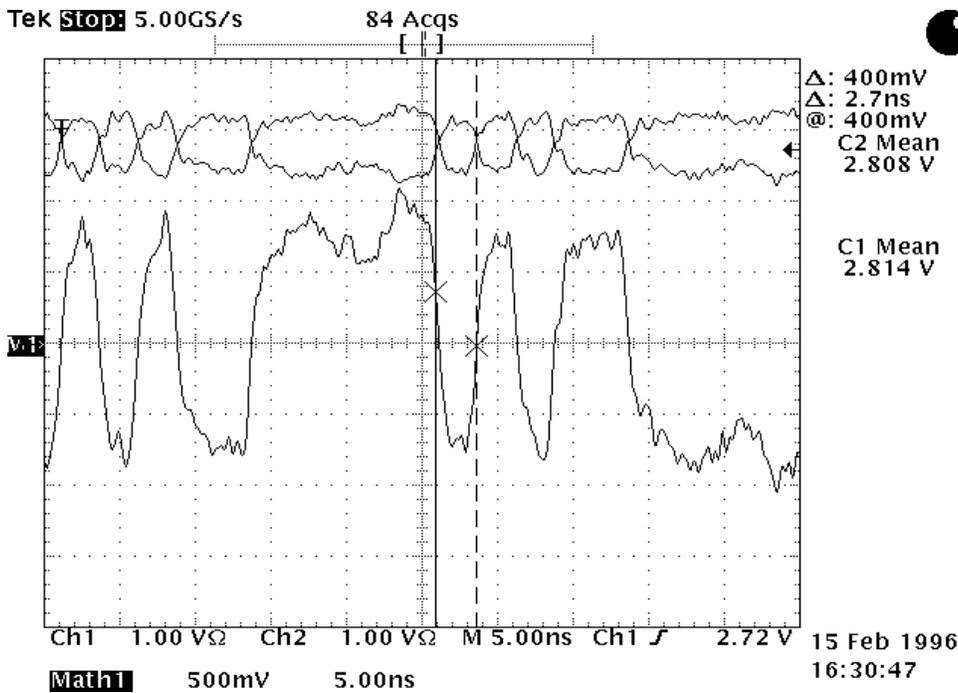
Figure 12: SSA Waveform: 40MB/s, single trigger, 2.0 meter cable
