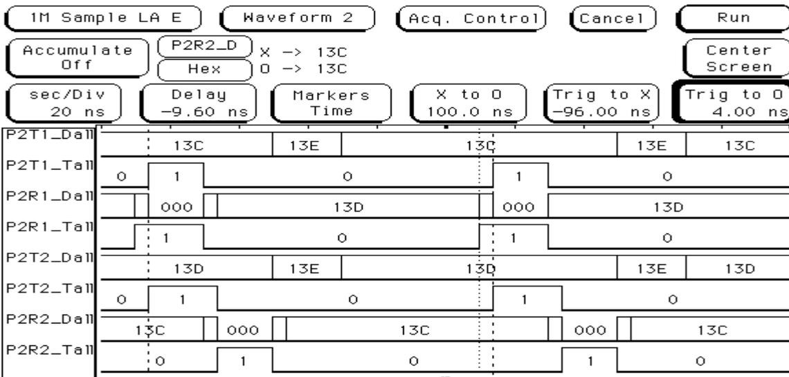
Figure 8: Protocol Waveform: 40MB/s normal mode synchronized
