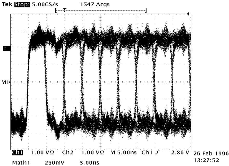
Figure 19: SSA RX Eye Diagram: 20MB/s, 0.6 meter cable
