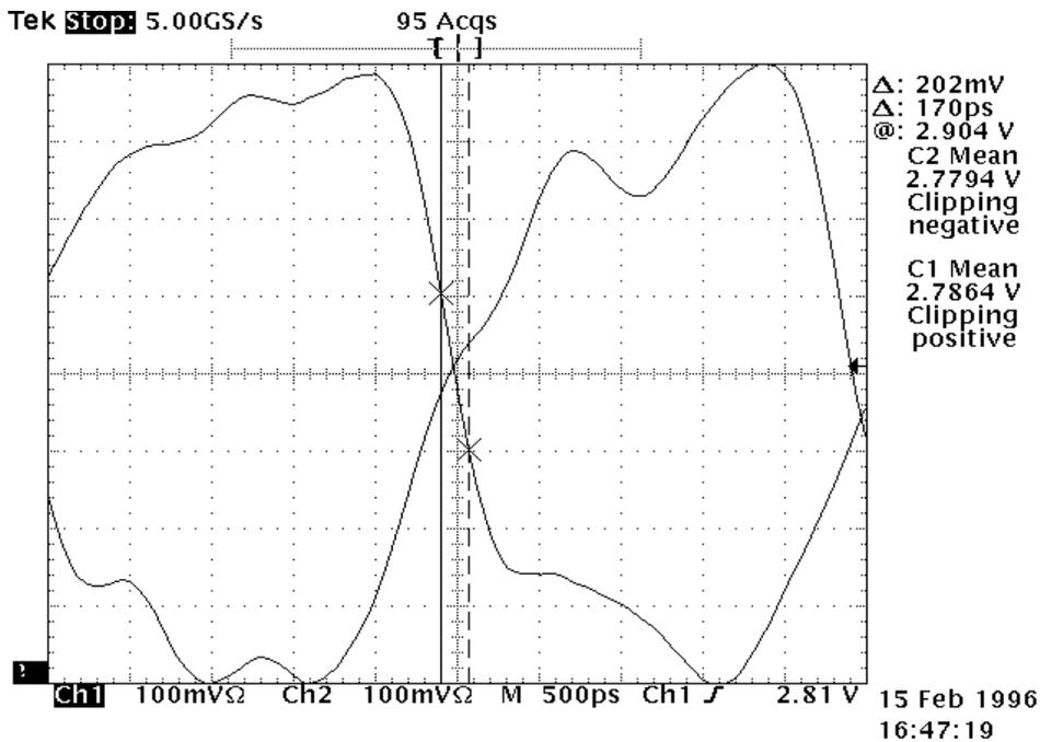
Figure 15: SSA Waveform: 40MB/s, fall time, 2.0 meter cable
