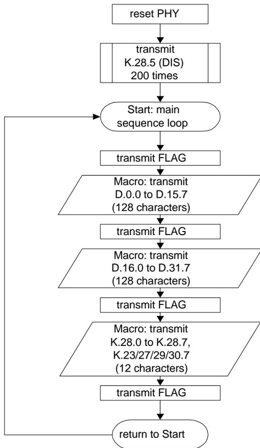
Figure 18: Transmit Pattern Sequence for Eye Diagrams
