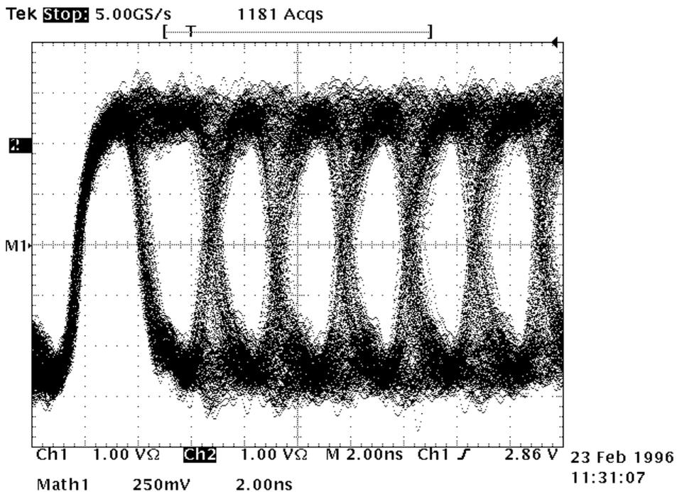
Figure 24: SSA RX Eye Diagram: 40MB/s, 2.0 meter cable
