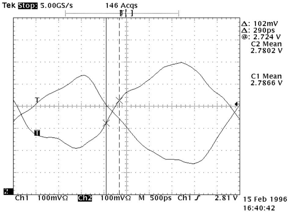
Figure 16: SSA Waveform: 40MB/s, rise time, 20.0 meter cable
