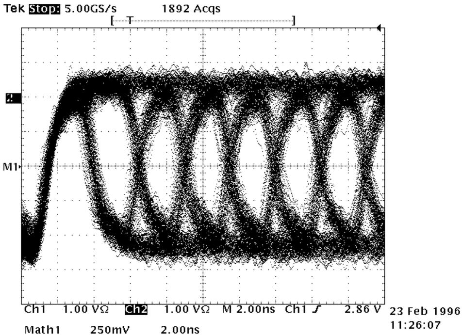
Figure 25: SSA RX Eye Diagram: 40MB/s, 10.0 meter cable
