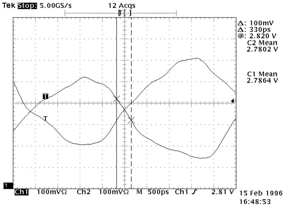
Figure 17: SSA Waveform: 40MB/s, fall time, 20.0 meter cable
