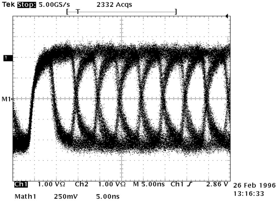
Figure 21: SSA RX Eye Diagram: 20MB/s, 20.0 meter cable
