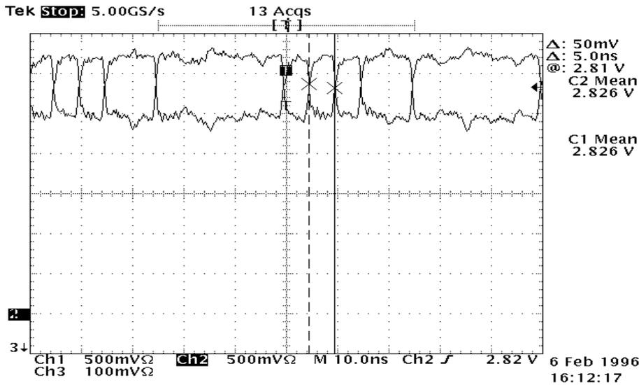
Figure 10: SSA Waveform: 20MB/s, single trigger, 2.0 meter cable
