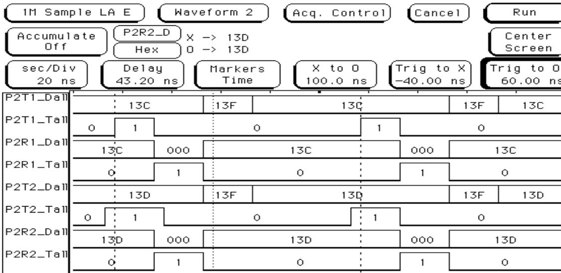
Figure 6: Protocol Waveform: 40MB/s wrap mode synchronized
