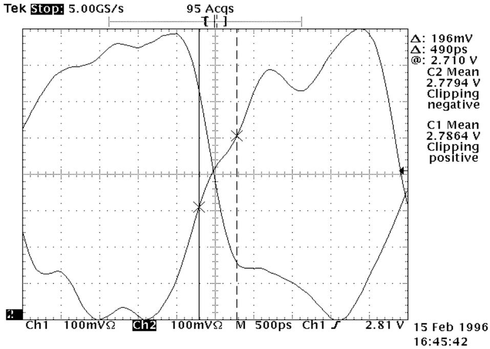
Figure 14: SSA Waveform: 40MB/s, rise time, 2.0 meter cable
