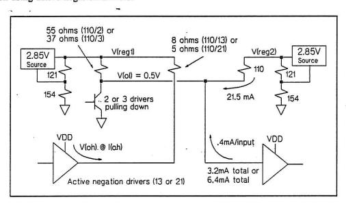
Consider the case of multiple signals driving high and one wired-OR signal driving low. The equivalent circuit for this is shown above. Assuming the active negation drivers all drive to V(oh) into their termination resistors, they have the potential to alter the regulator voltage.
