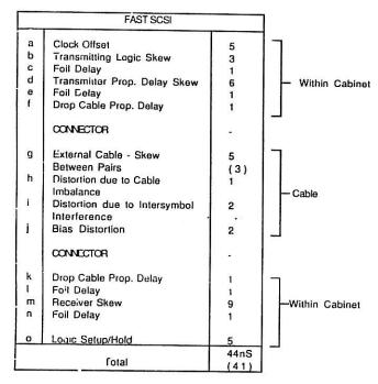
The numbers in parentheses are for a special cable Madison Cable is building for IPI use. It can also be used for SCSI.
