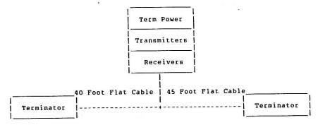
With this setup, driving MSG and C/D differentially, and leaving SEL undriven, TTL SEL received a 110 ns glitch (see photo). With cable lengths of 20 feet and 20 feet, TTL SEL had a 50 ns glitch (no photo). With cable lengths of 5 feet and 7 feet there was no TTL glitch.
