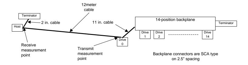
Equip: TDS794 with P6247(1GHZ) and P6246(400mhZ) probes
