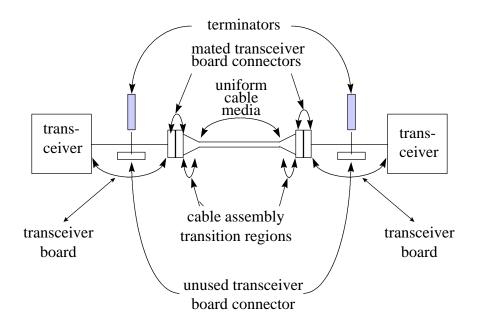
Figure 3 - Relationship of point to point SCSI connection components
