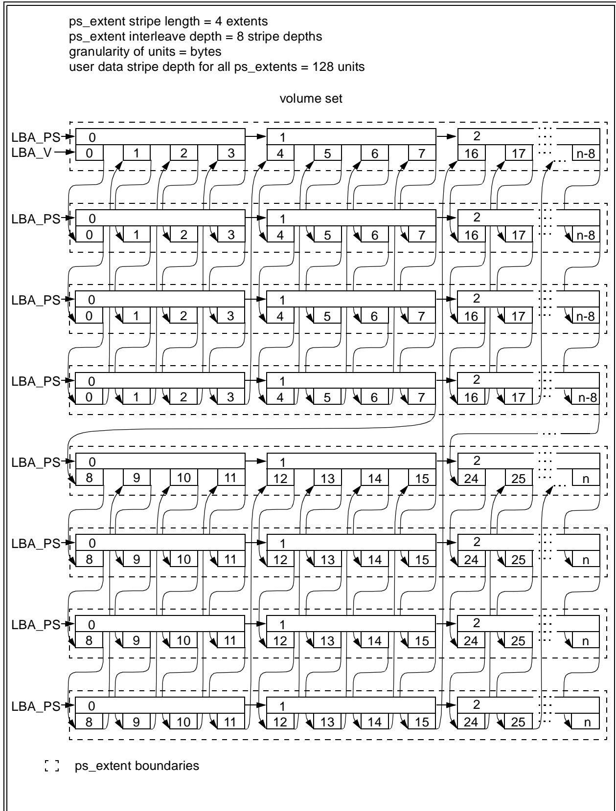
Figure C.5 - User data mapping for a RAID 3 configuration
