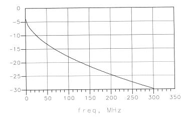
Note: The use of an attenuator for measuring shorter lengths is not acceptable because there is still mismatch loss uncertainty due to the fact that the attenuator does not have any better match than the far end test port. Also you introduce an additional uncertainty because you are trying to separate a small value ( cable attenuation ) from a large value, ( attenuator attenuation ) and you will face dynamic range issues. 5.3.2 Test Fixture Reference: 2.1.1.2 for appropriate test fixtures
