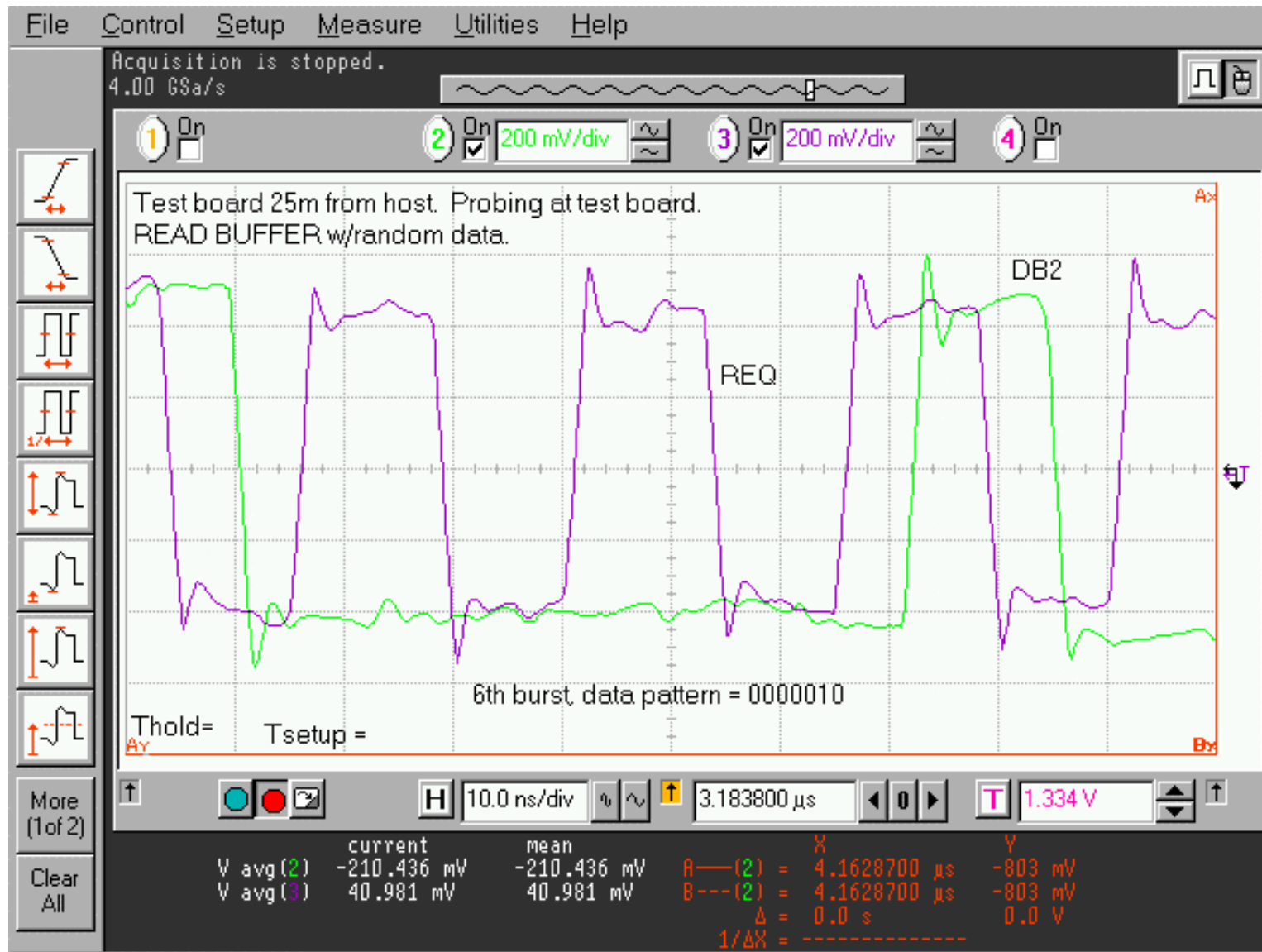
Slide 9: A single one after five zeroes, at target end. Should generate ISI condition at host end.
