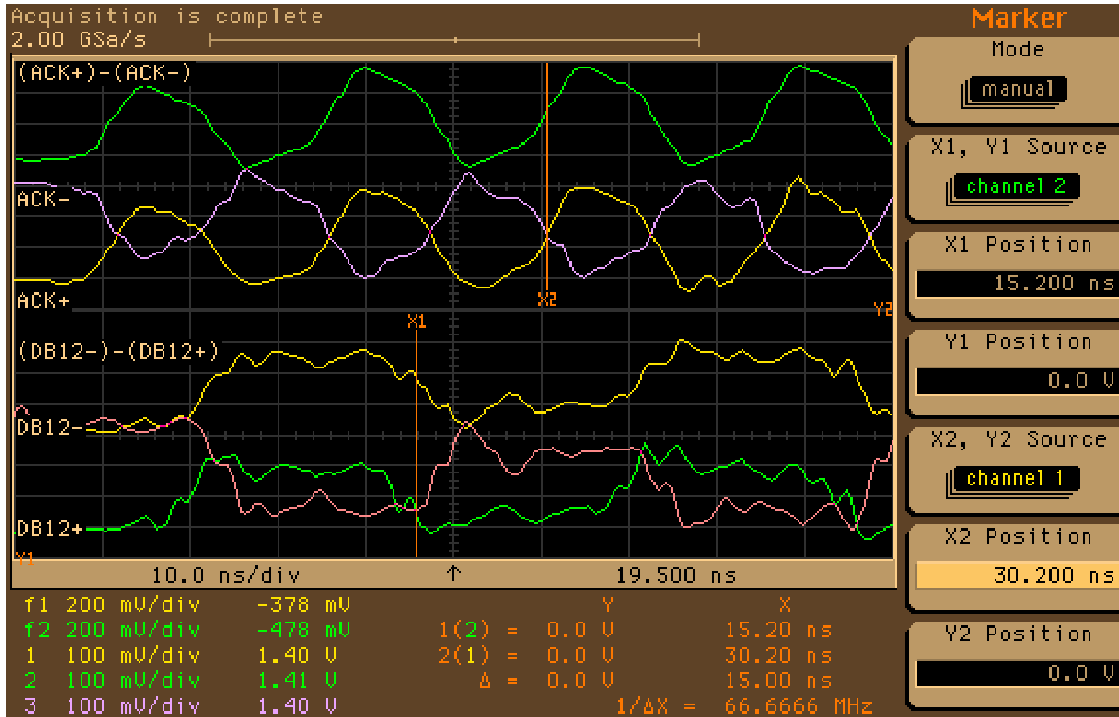
3.4pF graph, Write, data taken at the drive, position C
