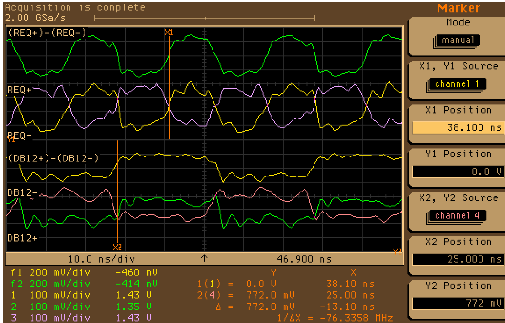
3.4pF graph, Read, data taken at the HBA, reading from position C
