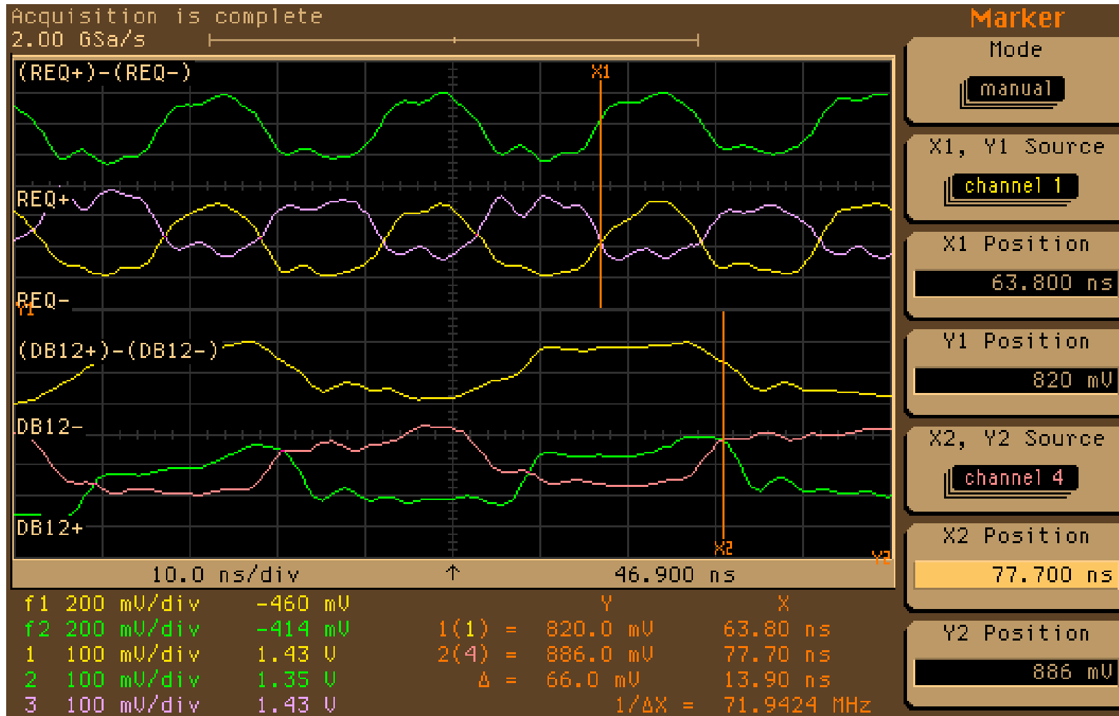
3.4pF graph, Read, data taken at the HBA, reading from position B
