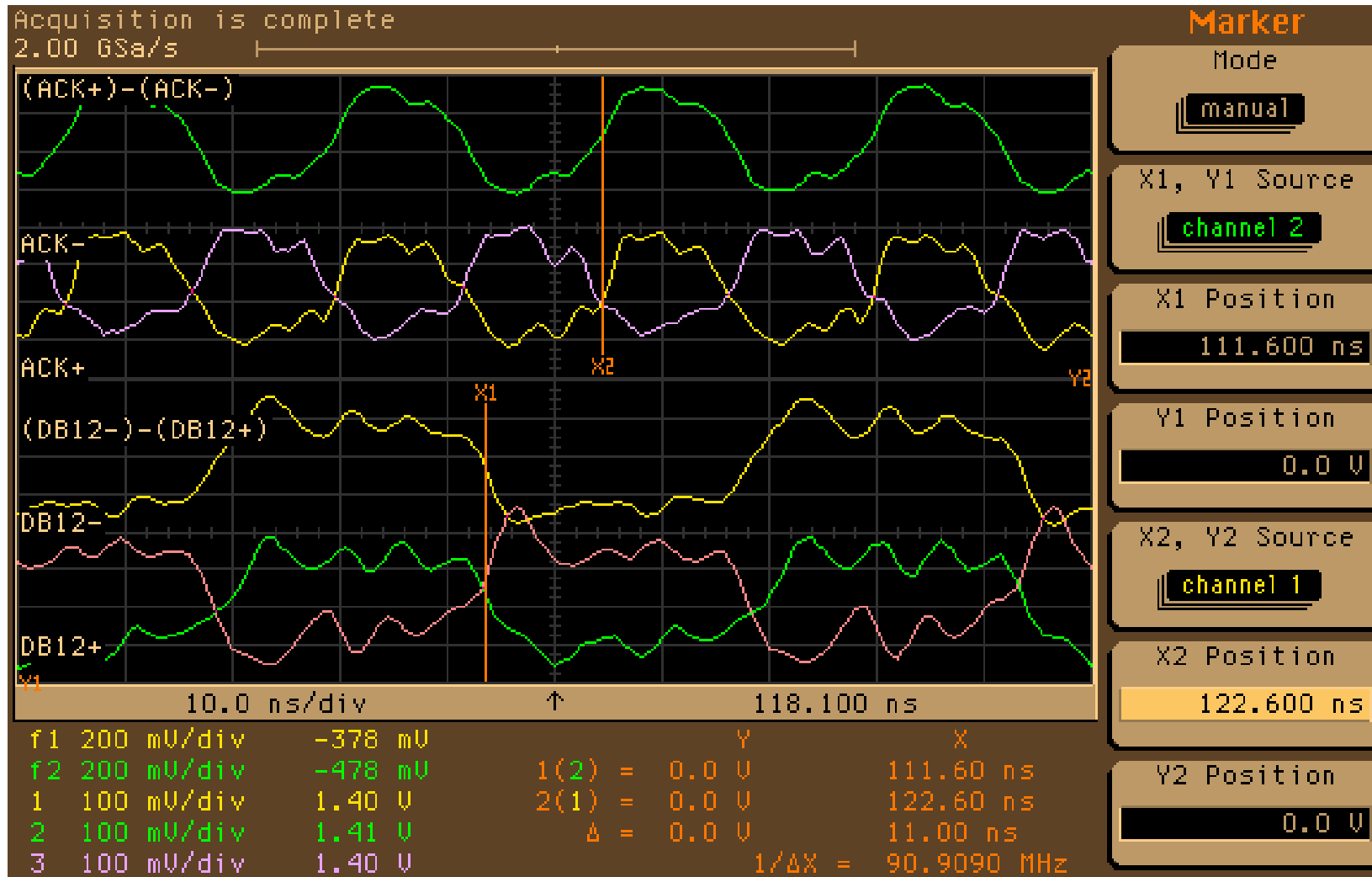
3.4pF graph, Write, data taken at the drive, position A
