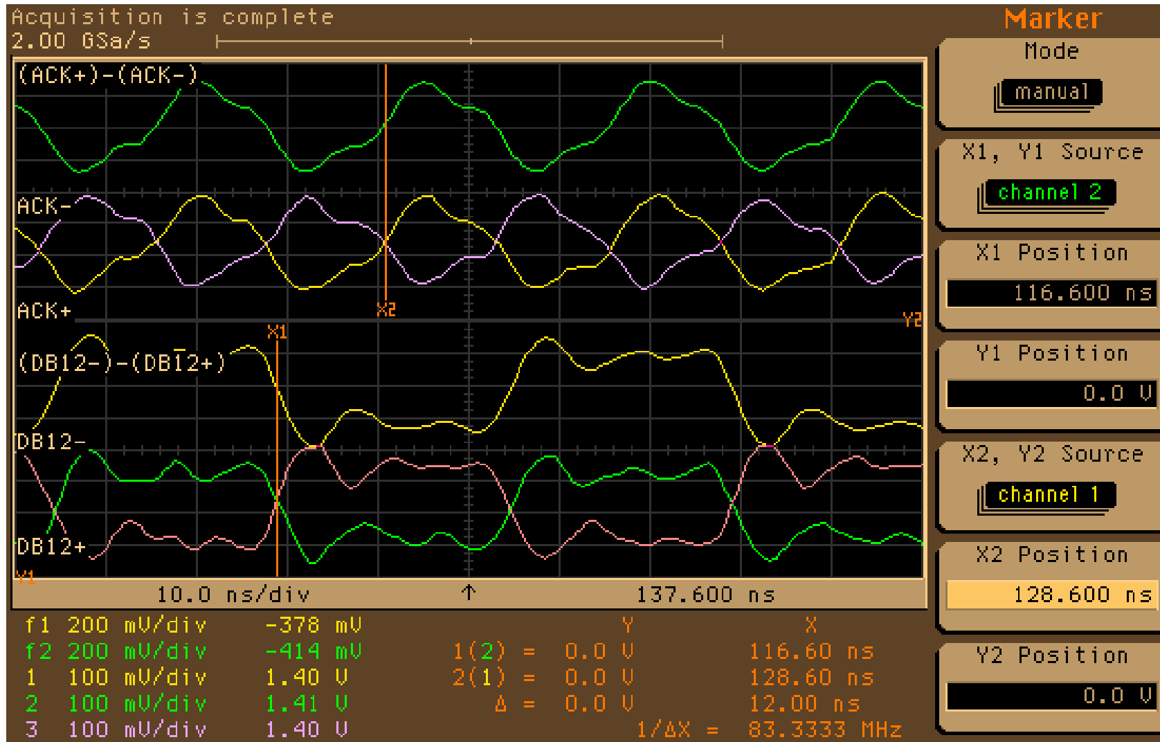
OpF graph, Write, data taken at the drive, position B
