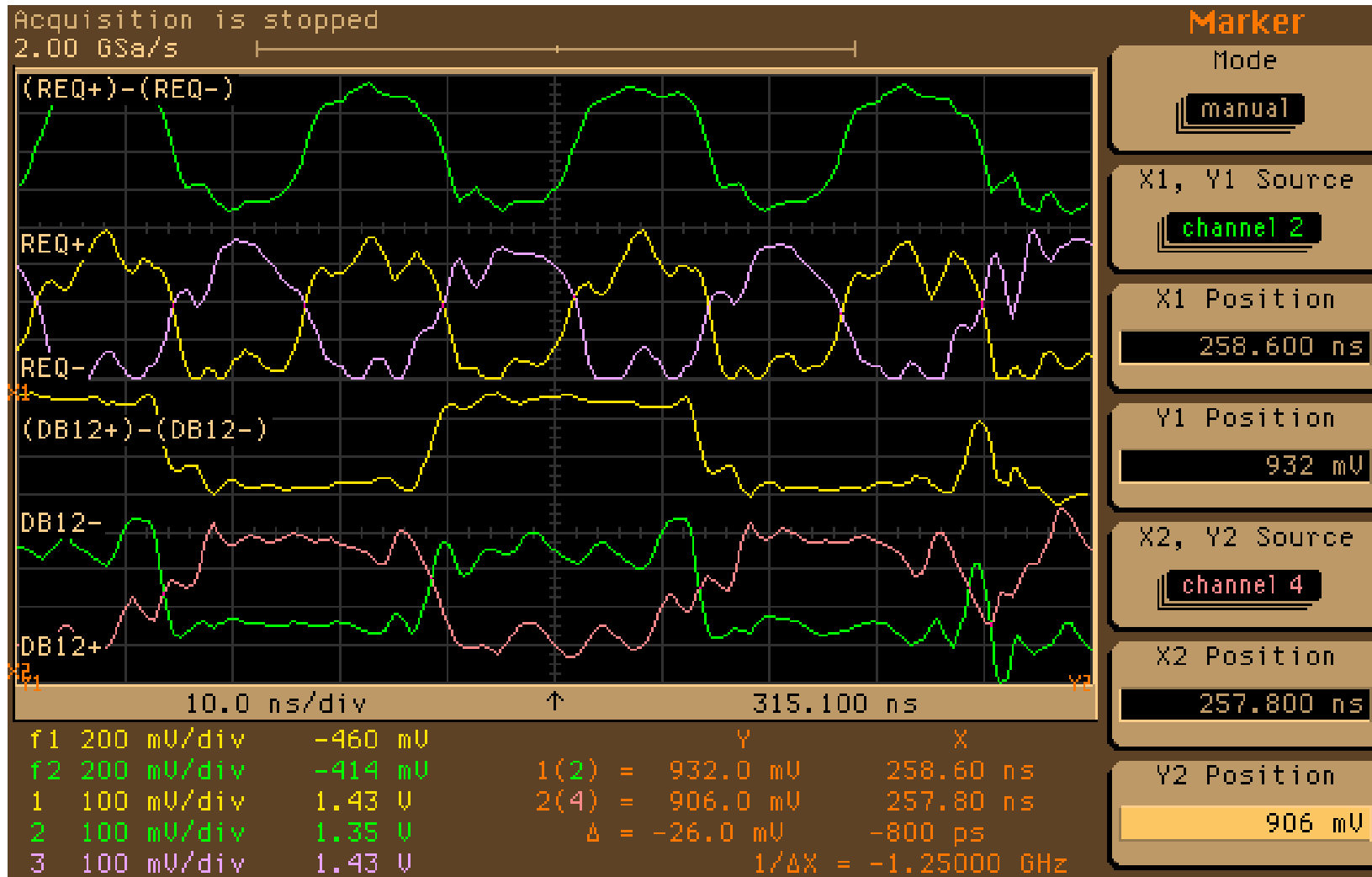
3.4pF graph, Read, data taken at the HBA, reading from position C, Competitor's drive (Note double clocking concern)
