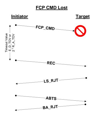
At this point the Initiator knows that the FCP\_CMD was not received at the target, and cannot be received by it in the future. It is up to the initiator to reissue the command.
