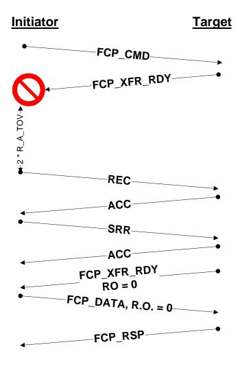
ACC for REC indicates that initiative was transferred to the initiator, but that the exchange is still open. The SRR requests retransmission of the FCP\_XFER\_RDY by R\_CTL setting in request. Target transmits FCP\_XFER\_RDY with RO of 0. Initiator transmits data.
