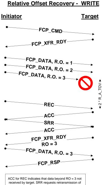
received by target. SRR requests retransmission of the FCP\_XFER\_RDY by R\_CTL setting in request. Target transmits FCP\_XFER\_RDY with RO and transfer count for data it didn't receive. Initiator retransmits lost data.
