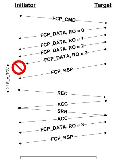
ACC for REC indicates that data beyond RO = 3 was sent by the target; initiator did not receive this. SRR requests retransmission of data from RO = 3 by setting solicited data as the R\_CTL. The target retransmits the data and response.
