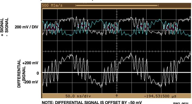
DUE TO ONLY ONE BIASING TERMINATION BEING USED
