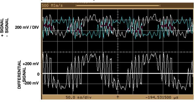
NOTE: DIFFERENTIAL SIGNAL IS OFFSET BY ~50 mV DUE TO ONLY ONE BIASING TERMINATION BEING USED
