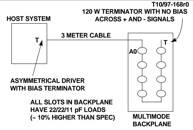
(MUST USE EXPANDER ON BACKPLNAE FOR THIS CONFIG) DATA AT A0, FAST 80 RATES, WORST CASE DATA PATTERN
