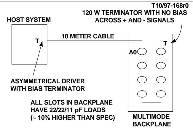
(MUST USE EXPANDER ON BACKPLANE FOR THIS CONFIG) DATA AT A0, FAST 80 RATES, WORST CASE DATA PATTERN
