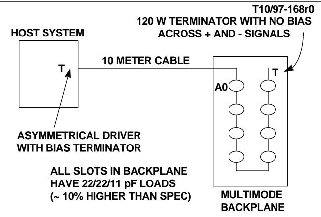
(SHOULD USE EXPANDER ON BACKPLANE FOR THIS CONFIG) DATA AT A0, FAST 40 RATES, WORST CASE DATA PATTERN
