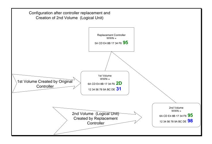
Note: The 2nd volume created is created with the WWN that is based on a value provided by the new controller. In this case, it is the new controller's WWN.
