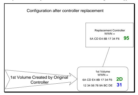
Note: The Volume continues to have the same WWN that was created with the original controller! This is absolutely required so that the volume can be correctly found by the system(s).
