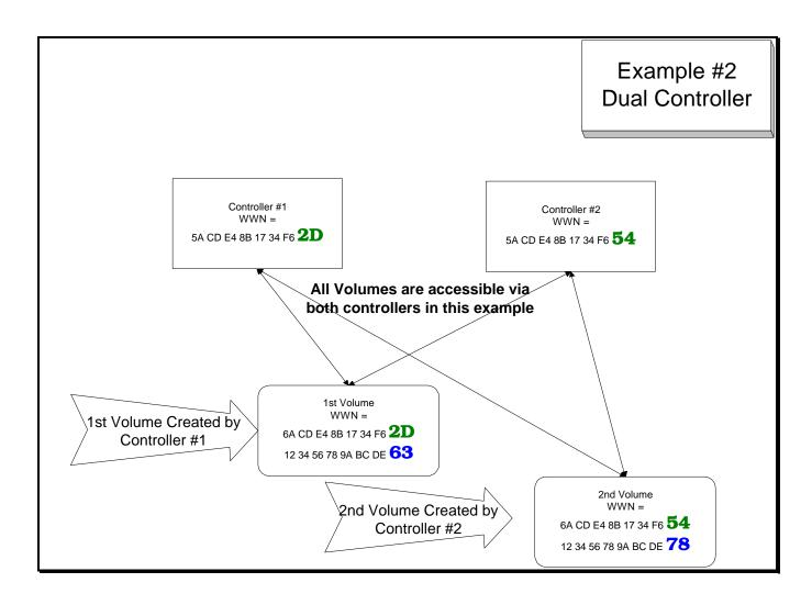
Note: Each Volume has the same WWN regardless of the path (controller) that it is accessed through. Furthermore, if either controller #1 or controller #2, the WWN for these volumes must NOT be changed.
