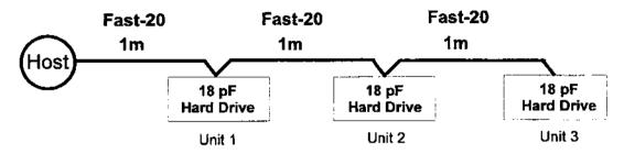
• Configuration: Test Case A - using three identical 18 pF hard disk drives
