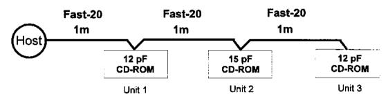
• Configuration: Test Case A - using three CD-ROM drives
