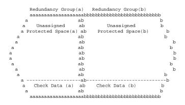
The following figure shows the relationship between check data, user data and protected space after a single volume set has been defined across the two redundancy groups.
