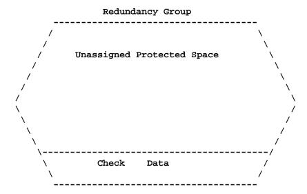
The following figure shows the relationship between the check data and protected space after two volume sets have been defined within the redundancy group.
