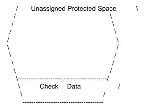
The following figure shows the relationship between the check data and protected space after two volume sets have been defined within the redundancy group.
