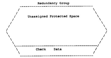
The following figure shows the relationship between the check data and protected space after two volume sets have been defined within the redundancy group.
