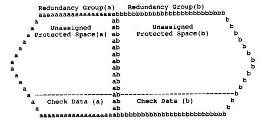
The following figure shows the relationship between check data, user data and protected space after a single volume set has been defined across the two redundancy groups.
