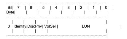
The IDENTIFY message is sent by either the initiator or the target to establish an I\_T\_L nexus. For dual port implementations: if the target disconnects from the bus during an I/O process, it shall reconnect through the same port when the I/O process is continued.
