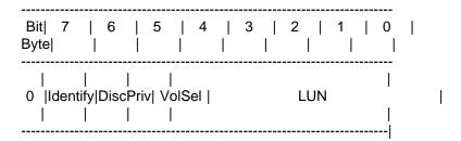
The IDENTIFY message is sent by either the initiator or the target to establish an I\_T\_L nexus. For dual port implementations: if the target disconnects from the bus during an I/O process, it shall reconnect through the same port when the I/O process is continued.
