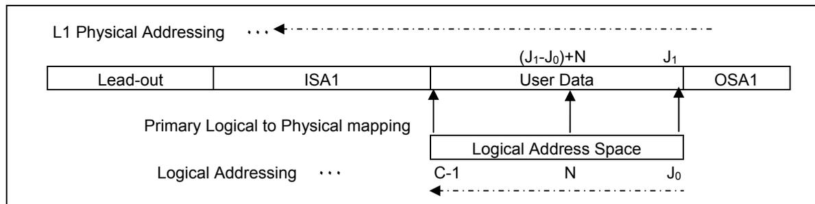
**Figure 16 — Logical to Physical Addressing on Layer 1**
