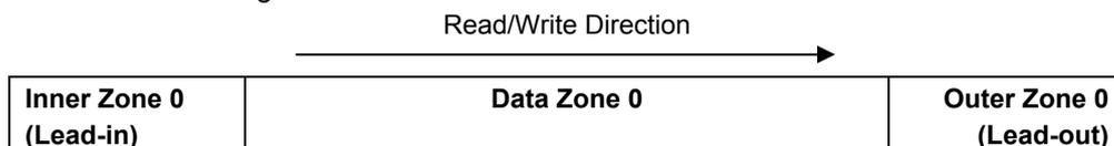
**Figure 2 — Primary Zones of a Single Layer BD disc**
