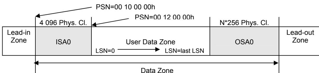
**Figure 6 — Layout of Single Layer BD-RE Disc**
