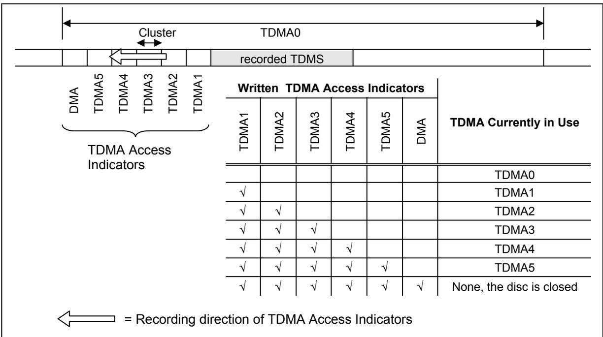
Figure 14 — TDMA Access Indicators on Dual Layer Disc
