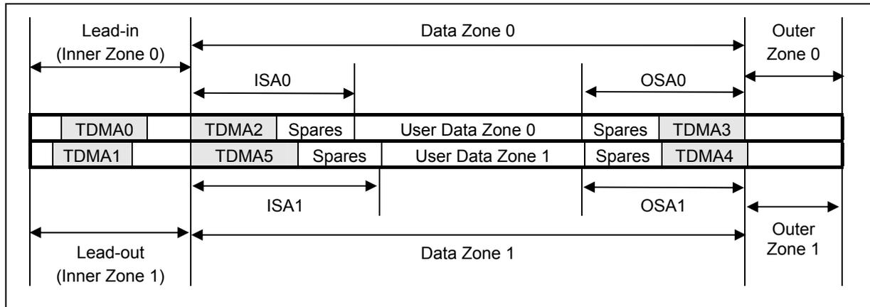
**Figure 12 — TDMA Allocation on DL BD-R**
