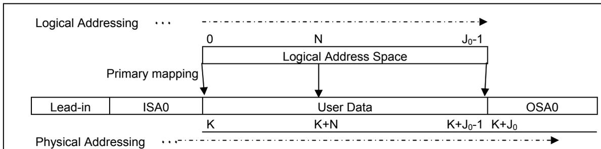
**Figure 15 — Logical to Physical Addressing on Layer 0**
