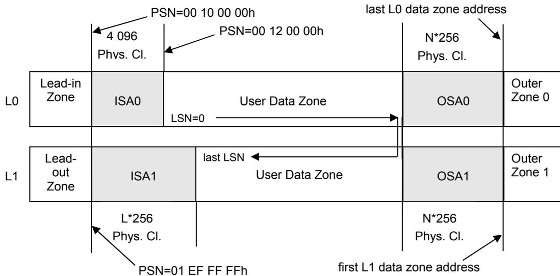
Figure 7 — Layout of Dual Layer BD-RE Disc
