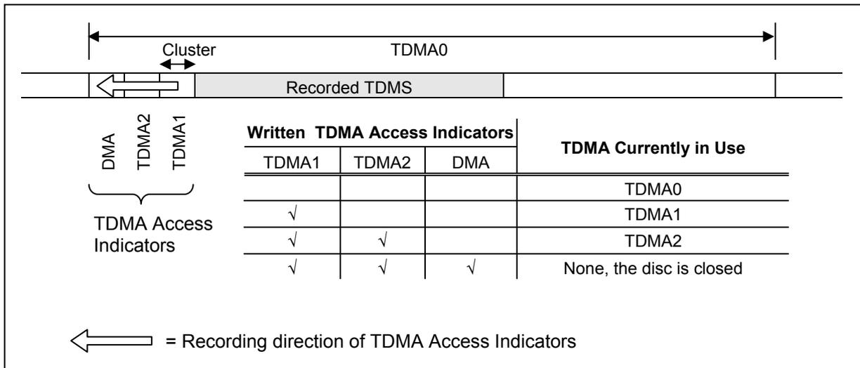
Figure 13 — TDMA Access Indicators on Single Layer Disc
