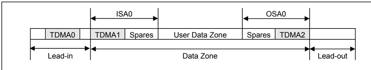
**Figure 10 — TDMA Allocation on SL BD-R**
