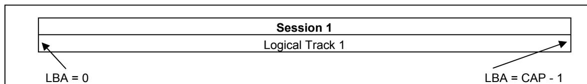
**Figure 17 — Status of a BD-R Disc After Formatting in SRM**
