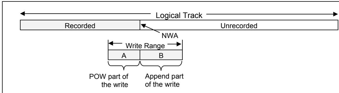
**Figure 30 — POW and Append Parts of WRITE**
