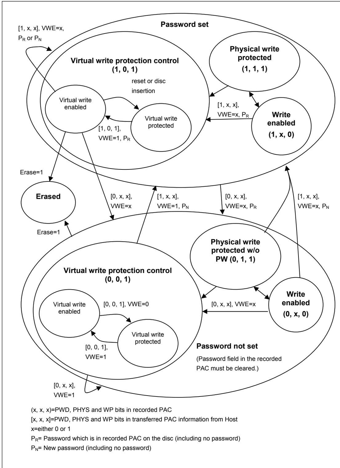
Figure 31 — Physical and Virtual Write Protect State Diagram
