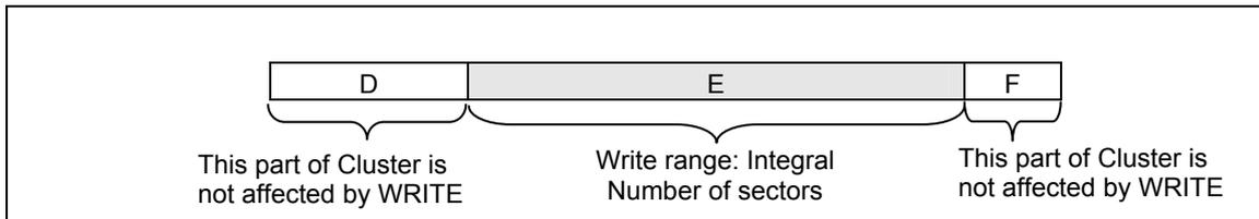
**Figure 29 — Parts of a POWed Cluster**
