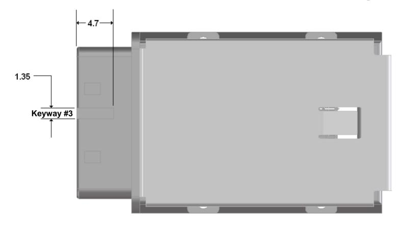
CAGE GASKET REMOVED FOR CLARITY TOLERANCE = +/-0.1MM
