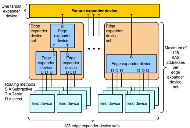
Figure 25 — Maximum expander device set topology
