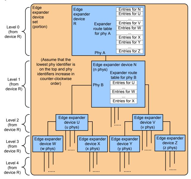
Figure 48 — Expander route index levels example
