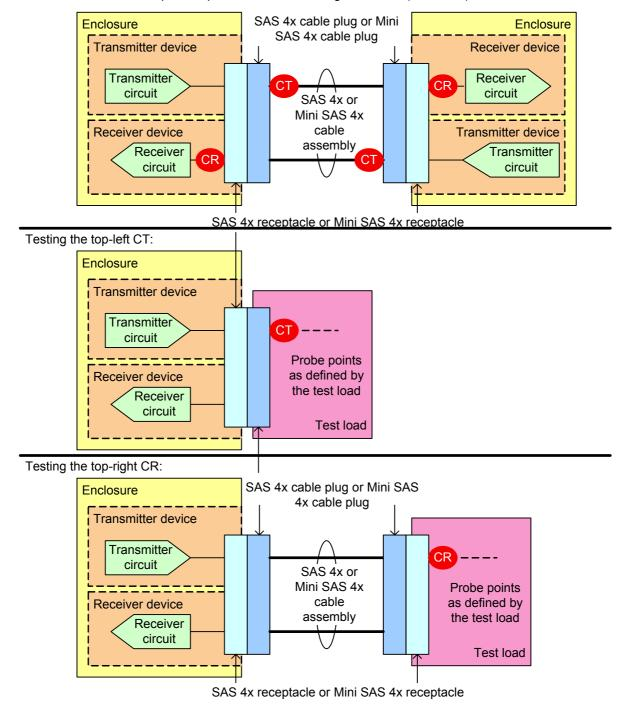
Figure 89 — SAS 4x and Mini SAS 4x cable assembly CT and CR compliance points
