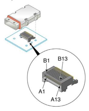
Figure 72 — Mini SAS 4x receptacle connector
