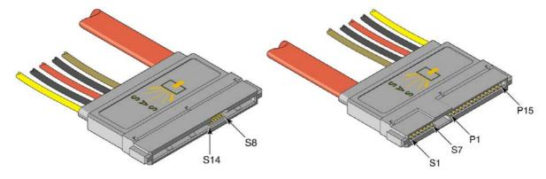
Figure 60 — Single-port SAS Drive cable receptacle connector
