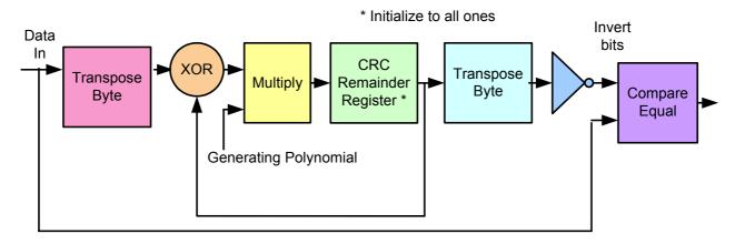
Figure D.2 — CRC checker example
