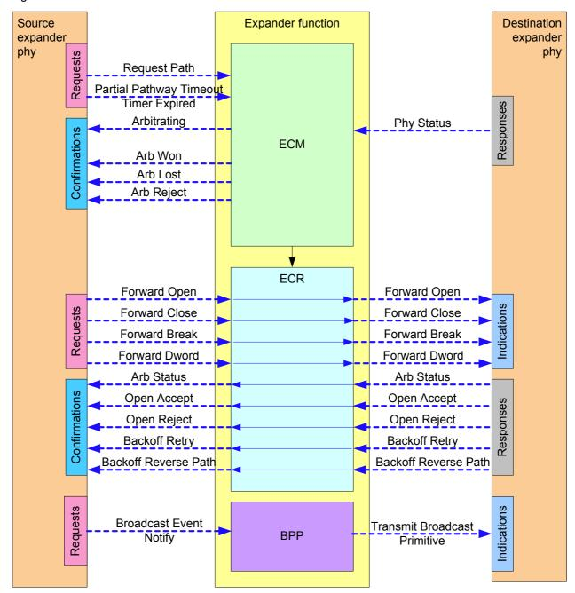
Figure 44 — Expander device interface detail
