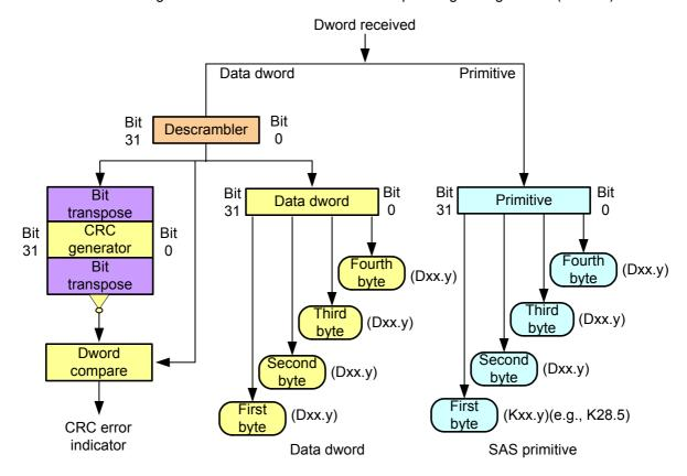
Figure 136 — Receive path bit ordering
