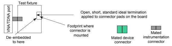
Figure B.4 — De-embedding of connectors in test fixtures
