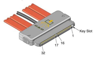
Figure 63 — SAS 4i cable receptacle connector
