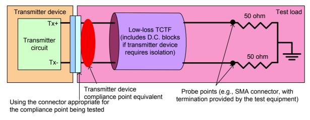
Figure 101 — Low-loss TCTF test load
