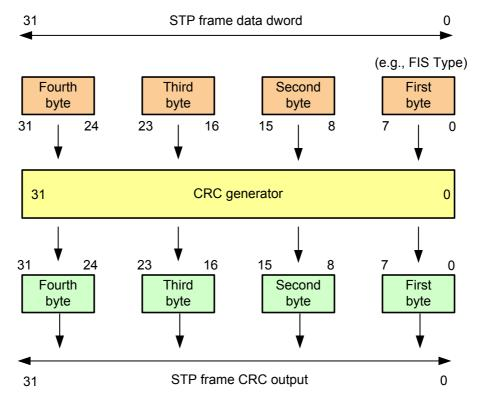
Figure 134 — STP frame CRC bit ordering
