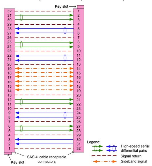
Figure 78 — SAS internal symmetric cable assembly - SAS 4i
