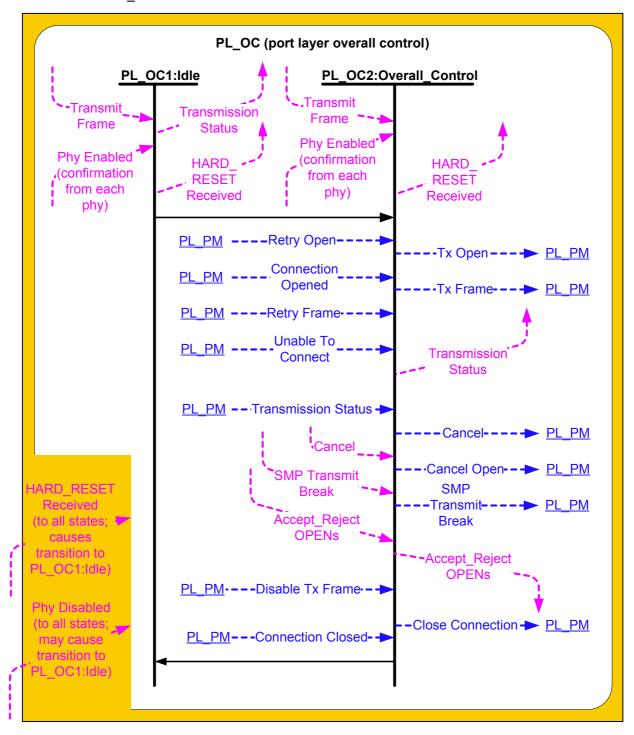
Figure 167 — PL\_OC (port layer overall control) state machine
