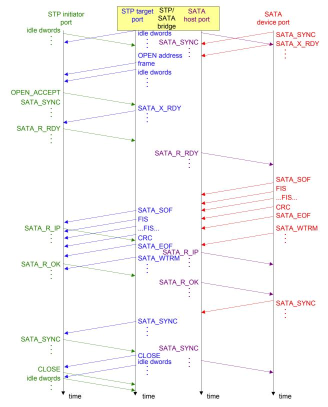
Figure 162 — STP target port opening an STP connection
