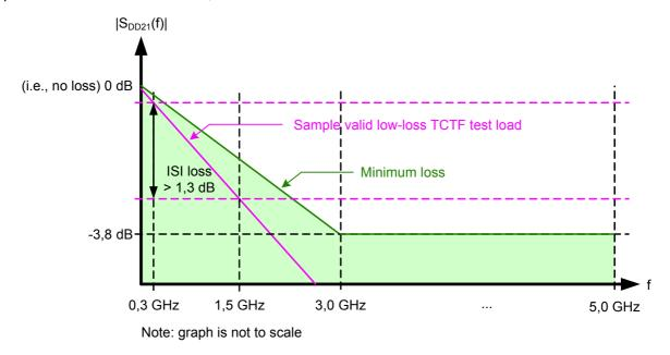
Figure 102 — Low-loss TCTF test load S<sub>DD21</sub> and ISI loss requirements at 3,0 Gbit/s
