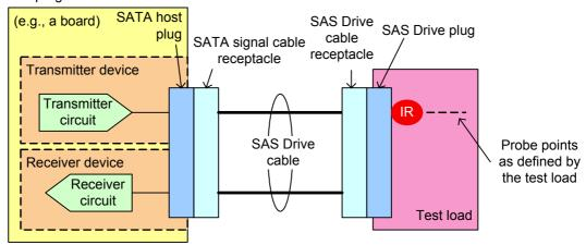
Figure 95 — Internal cable IT and IR compliance points
