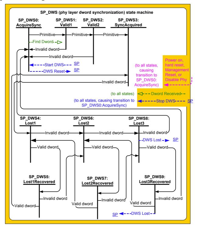
Figure 127 — SP\_DWS (phy layer dword synchronization) state machine
