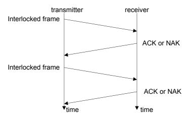
Figure 151 — Interlocked frames
