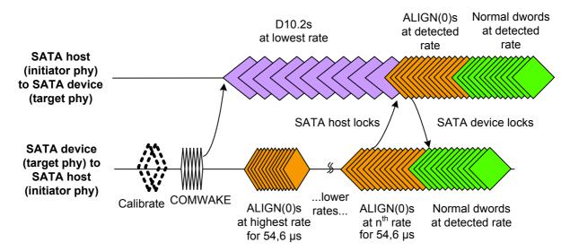
Figure 115 — SATA speed negotiation sequence
