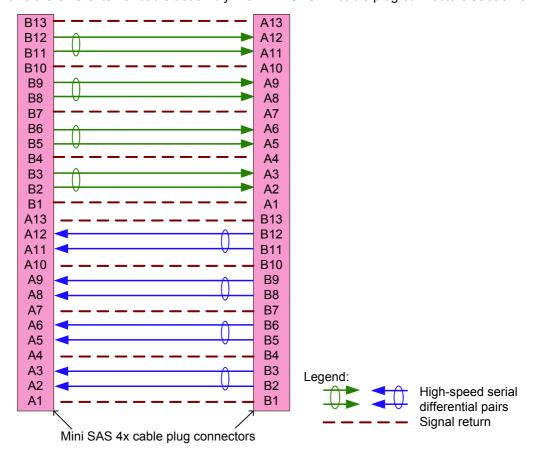
Figure 86 — SAS external cable assembly - Mini SAS 4x
