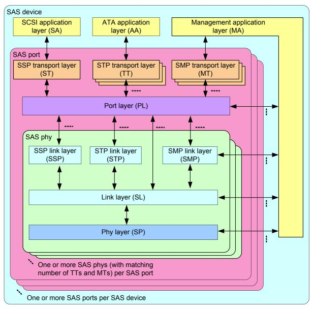
Figure 30 — State machines for SAS devices
