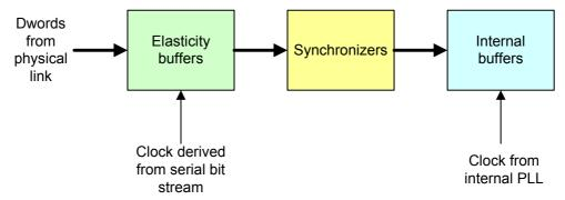
Figure 132 — Elasticity buffers
