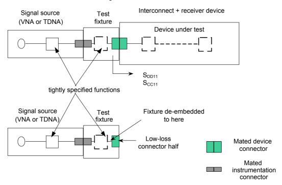
Figure B.17 — Measurement conditions for downstream return loss at IT or CT
