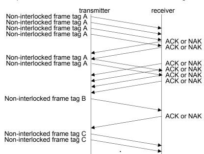
Figure 153 shows an example of non-interlocked frame transmission with different tags.
