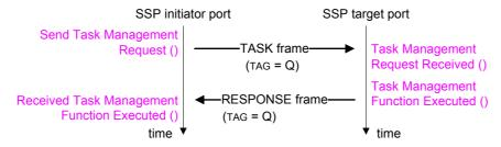
Figure 170 — Task management function sequence of SSP frames
