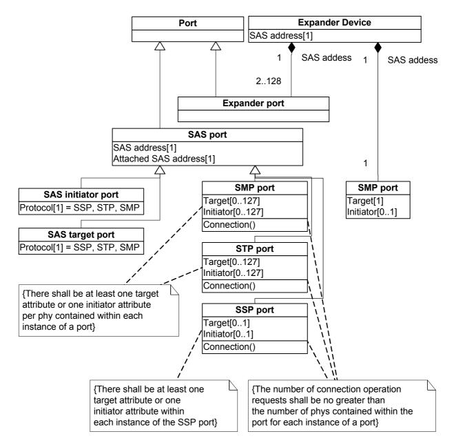
Figure 15 — Port class diagram
