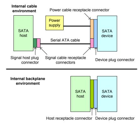
Figure 51 — SATA connectors and cables
