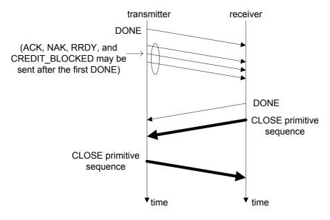
Figure 154 — Closing an SSP connection example
