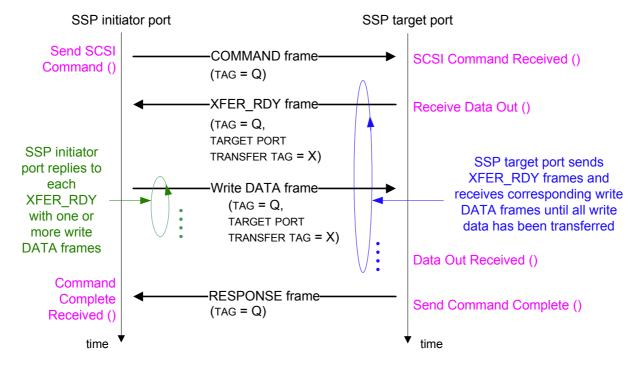
Figure 172 — Write command sequence of SSP frames
