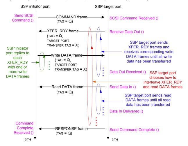
Figure 174 — Bidirectional command sequence of SSP frames
