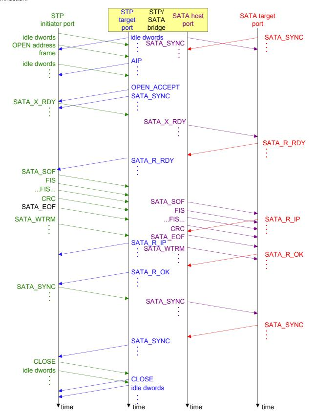
Figure 161 — STP initiator port opening an STP connection
