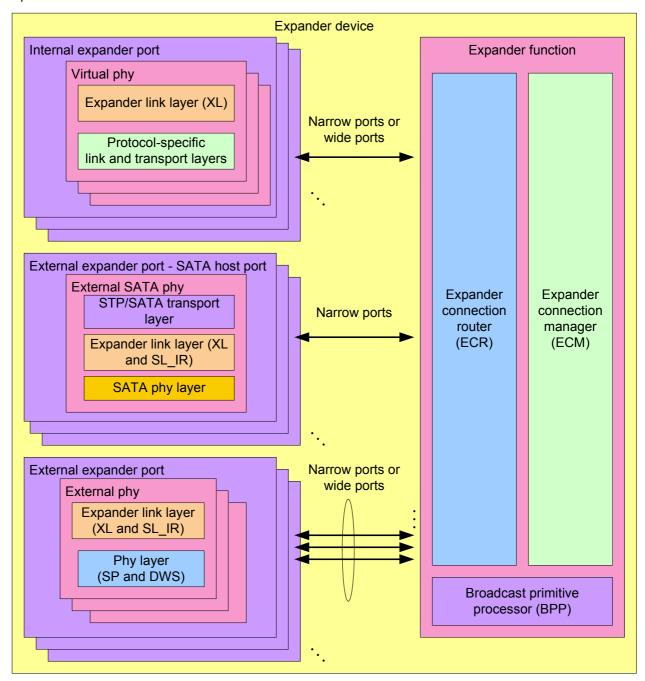
Figure 42 — Expander device model
