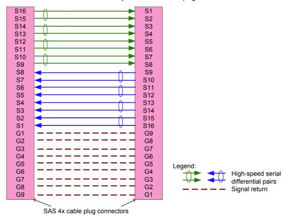
Figure 85 — SAS external cable assembly - SAS 4x
