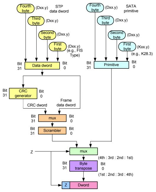
STP dword to transmit+data/primitive indicator (Z)
