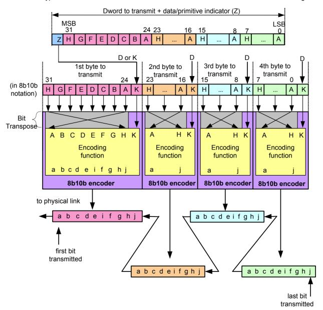
Figure 109 — SAS bit transmission logic
