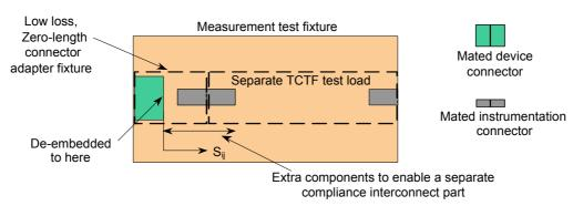
Figure B.6 — Transmitter device signal output measurement test fixture details
