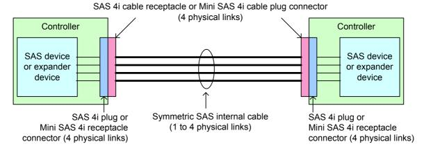
Figure 56 — SAS internal symmetric cable environment - controller to controller
