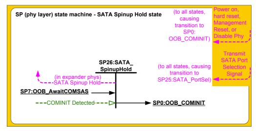
Figure 126 — SP (phy layer) state machine - SATA spinup hold state
