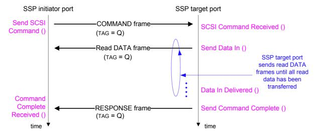
Figure 173 — Read command sequence of SSP frames
