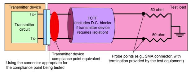
Figure 98 — TCTF test load
