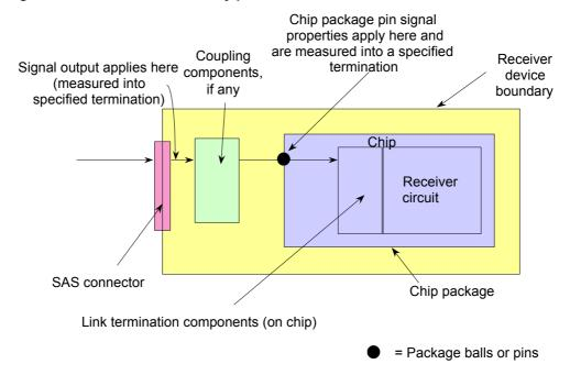
Figure B.3 — Receiver device details
