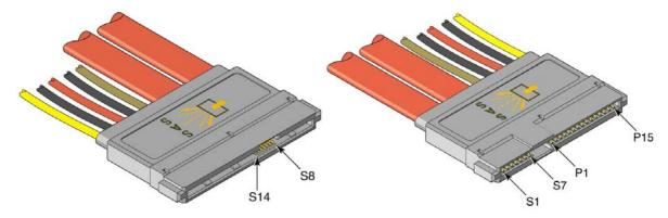
Figure 61 — Dual-port SAS Drive cable receptacle connector
