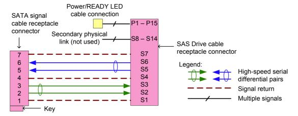
Figure 76 — Single-port SAS Drive cable assembly
