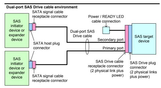
Figure 52 — SAS Drive cable environments
