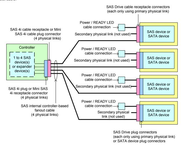
Figure 57 — SAS internal controller-based fanout cable environment
