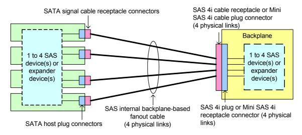
Figure 58 — SAS internal backplane-based fanout cable environment
