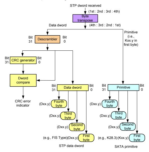
Figure 138 — STP receive path bit ordering
