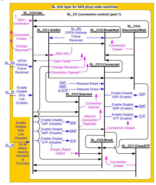
Figure 145 — SL (link layer for SAS phys) state machines (part 1)
