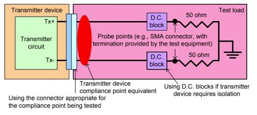
Figure 96 — Zero-length test load for transmitter device compliance point
