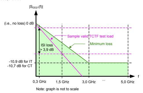
Figure 99 — TCTF test load S<sub>DD21</sub> and ISI loss requirements at 3,0 Gbit/s
