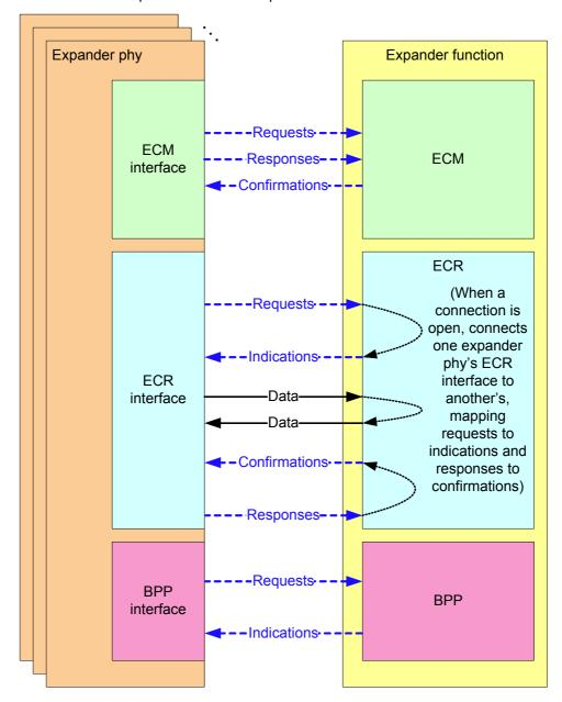
Figure 43 — Expander device interfaces
