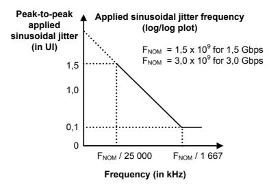
Figure 108 — Applied sinusoidal jitter
