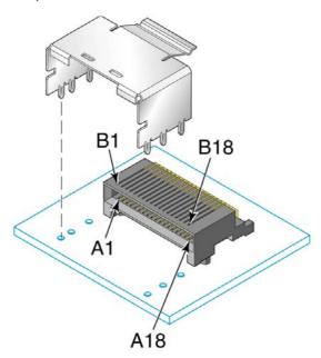
Figure 66 — Mini SAS 4i receptacle connector
