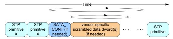
Figure 159 — Transmitting a continued primitive sequence
