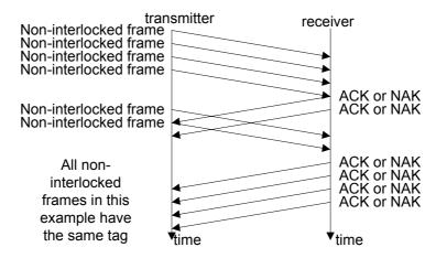
Figure 152 — Non-interlocked frames with the same tag
