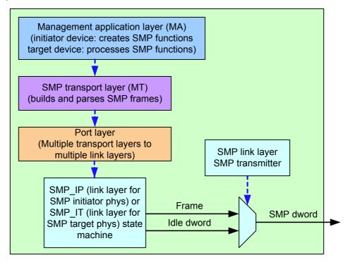
Figure 34 — SMP link, port, SMP transport and management application layer state machines
