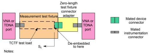
1 This is not identical to the measurement test fixture used for the transmitter output signal even though the connector genders are the same. The pins used in the SAS connector are for the Rx (i.e., not the Tx) signals and the signals flow the other way. The  $S_{22}$  measurement here is the same as the  $S_{11}$  measurement for the transmitter output signal but on different pins.
