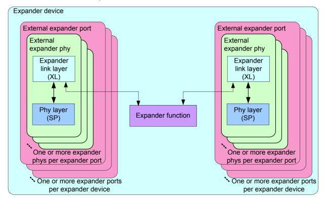
Figure 31 — State machines for expander devices
