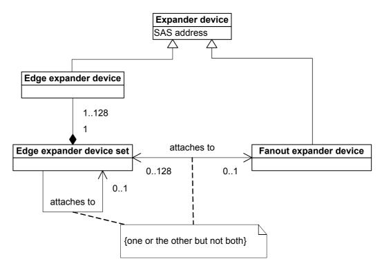
Figure 19 — Expander device class diagram
