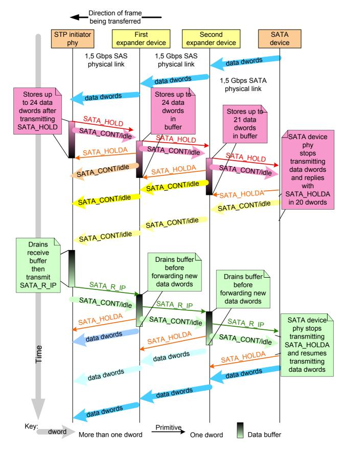
Figure 158 — STP flow control
