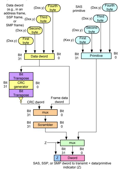
Figure 135 — Transmit path bit ordering
