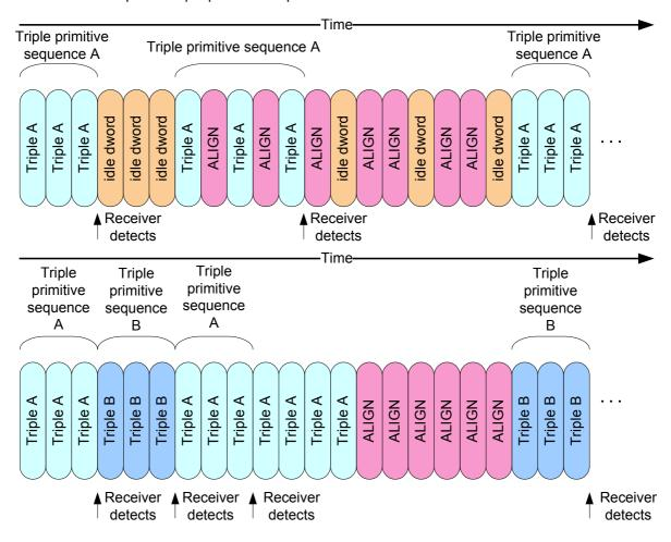
Figure 130 — Triple primitive sequence
