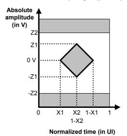
Figure 105 — Transmitter device eye mask
