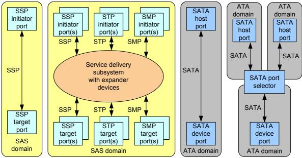
Note: When expander devices are present, SAS target ports may be located in SAS devices contained in expander devices.
