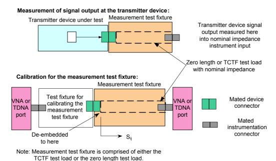
Figure B.5 — Measurement conditions for signal output at the transmitter device
