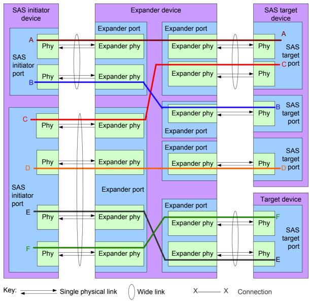
Note: The expander device has a unique SAS address. Each SAS initiator port and SAS target port has a unique SAS address. Connections E and F represent a wide SAS initiator port with two simultaneous connections to a wide SAS target port.
