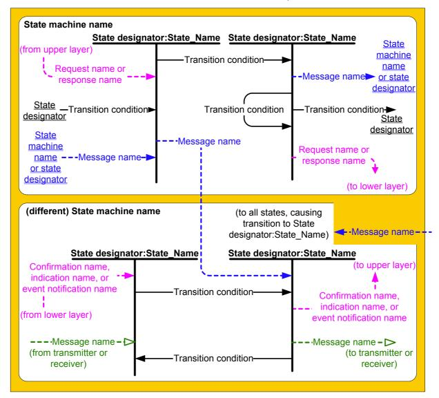
Figure 9 — State machine conventions
