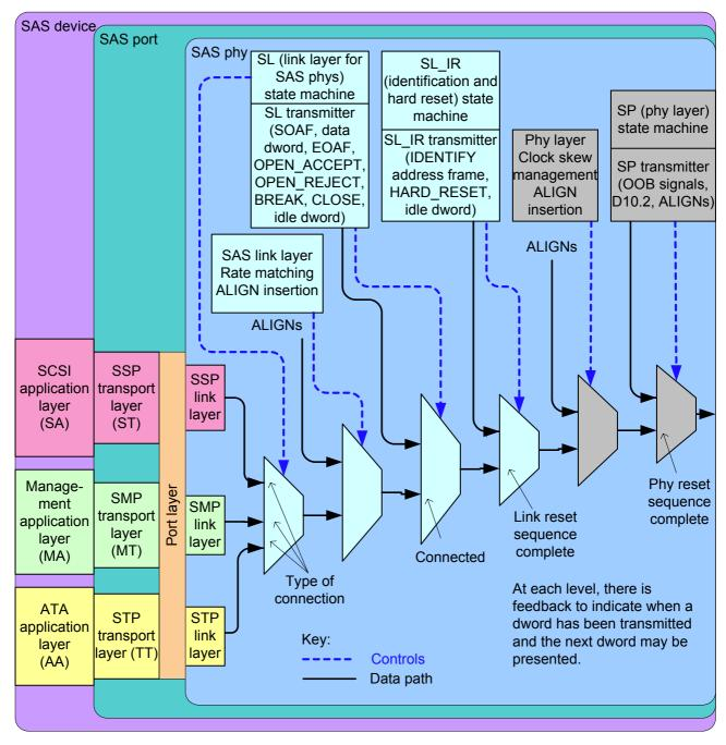
Figure 32 — Transmit data path in a SAS phy
