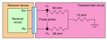
Figure 104 — Receiver device transient test circuit
