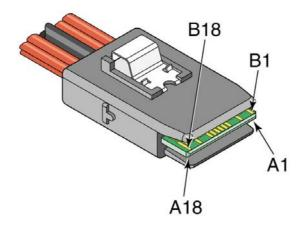
Figure 65 — Mini SAS 4i cable plug connector
