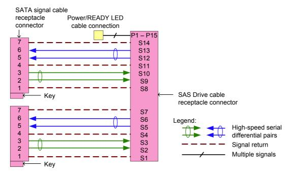
Figure 77 — Dual-port SAS Drive cable assembly
