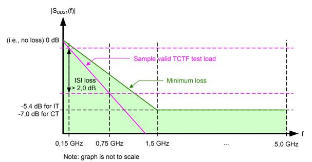
Figure 100 — TCTF test load S<sub>DD21</sub> and ISI loss requirements at 1,5 Gbit/s
