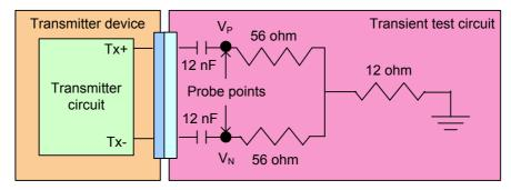
Figure 103 — Transmitter device transient test circuit
