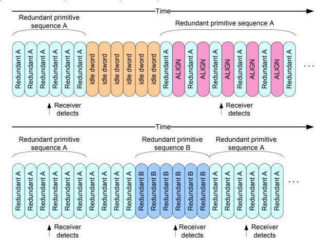
Figure 131 — Redundant primitive sequence
