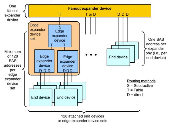
Figure 26 — Fanout expander device topology
