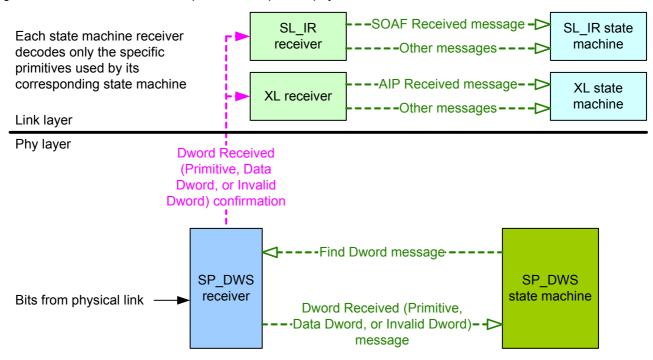
Figure 38 — Receive data path in an expander phy
