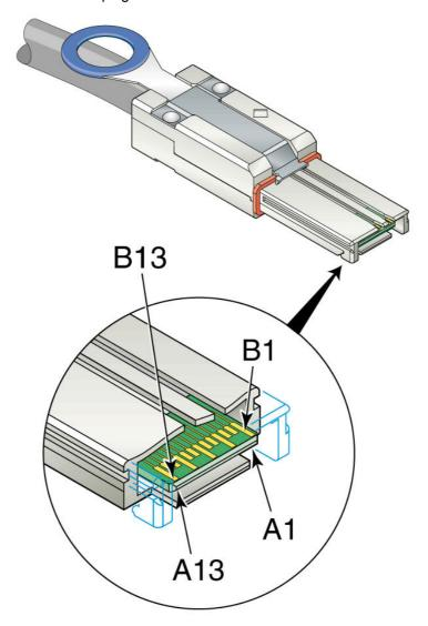
Figure 69 — Mini SAS 4x cable plug connector
