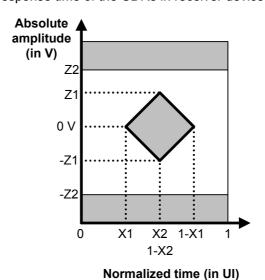
Figure 106 — Receiver device eye mask
