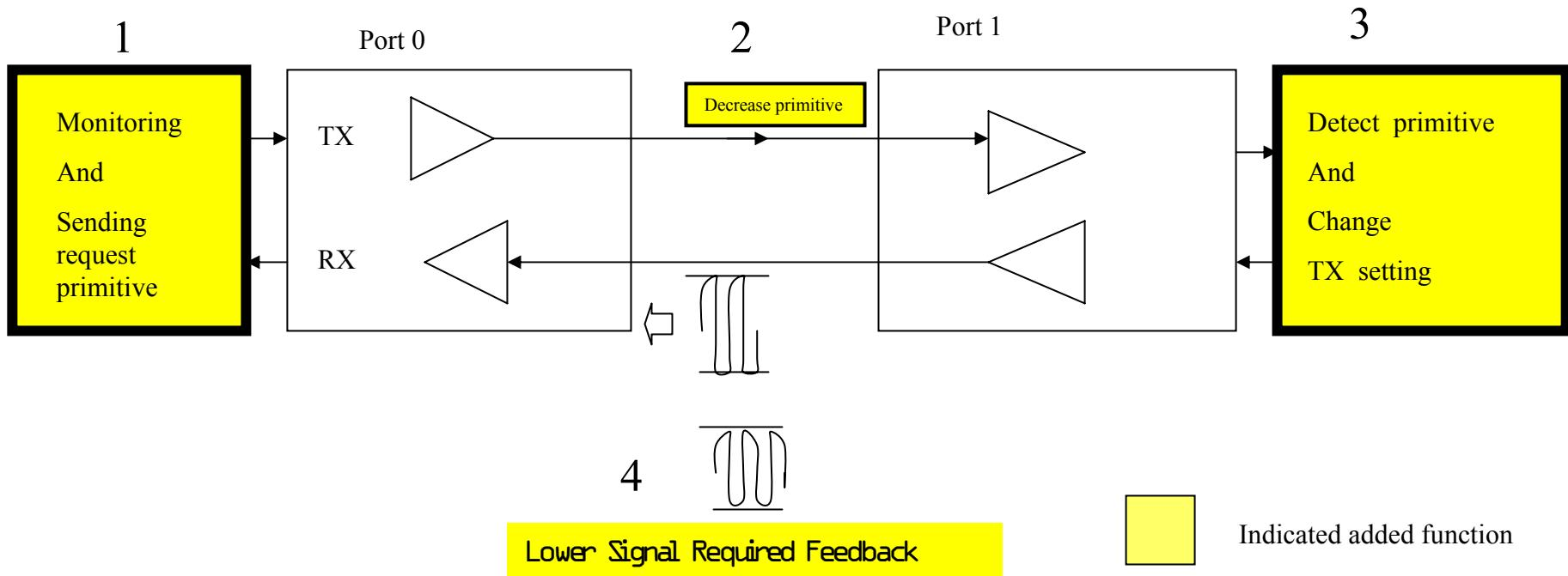
1. Port 0 RX : Monitoring & detecting over level of receiving signal
