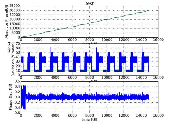
The jitter on the fundimental transmit signal is passed through a compliance CDR transfer function, to extract the high frequency sampling jitter.
