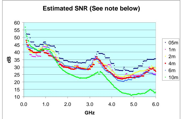
The crosstalk curves used to derive this estimate may include a resonance response. Frequencies where the resonances cancel out will still be problematic for digital signaling
