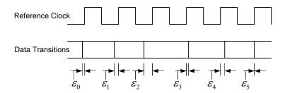
The response time of the PLL is in the microseconds because the bandwidth is in the megahertz. Over this time interval, thousands of bit transitions occur; hence the loop converges to a long term average. Over a time interval of tens of bits, the action of the PLL on the time deviations or error  $\mathcal{E}_k$  tends to simply average the error.
