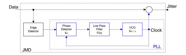
In response to jitter, the jitter transfer function is J(s) = 1 - H(s)
