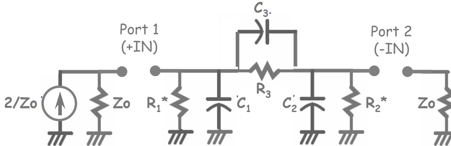
$$R_1 = R_1^* \parallel Z_0, \quad R_2 = R_2^* \parallel Z_0, \quad R_1 C_1 = R_2 C_2 = R_3 C_3 = \tau$$
