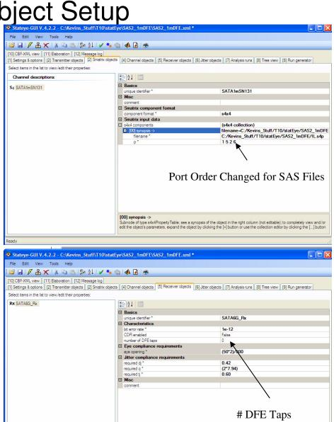
Parameter used to decide on eye opening compliance at the end of a complete analysis run: required vertical eye opening
