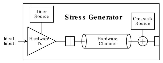
Calibration Suite (Method for testing the validity of the Stress Generator)
