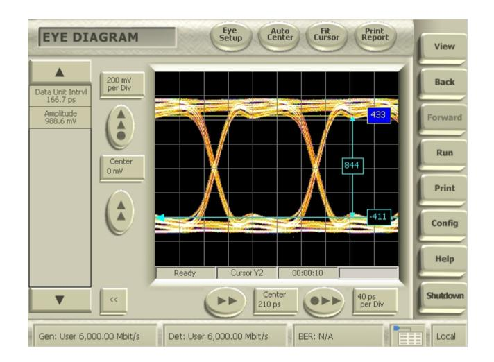
Eye Height Measured / Simulated: 844mV / 893mV
