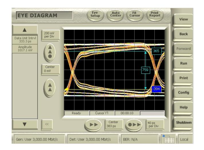
Eye Height Measured / Simulated: 759mV / 794mV
