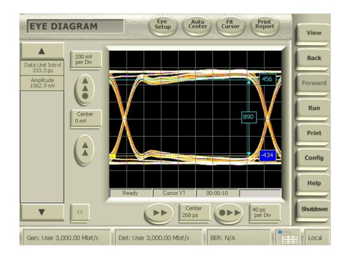
Eye Height Measured / Simulated: 890mV / 926mV
