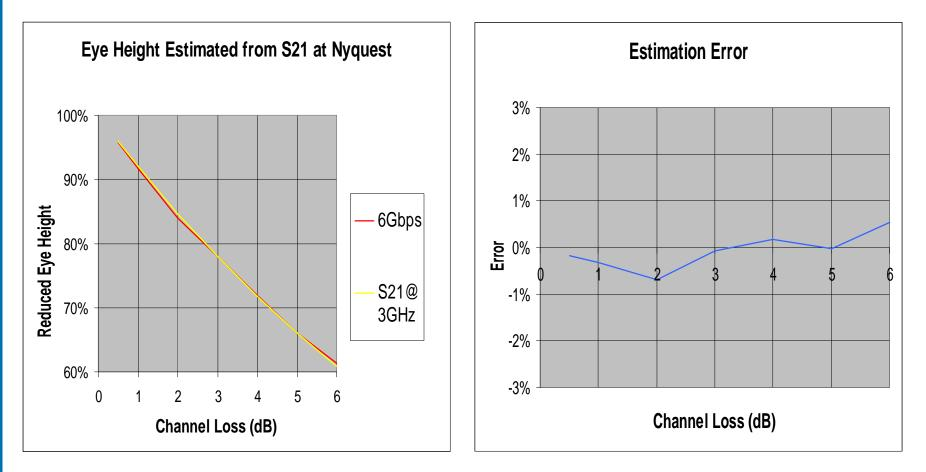
(Insertion Loss Measured at 3GHz)
