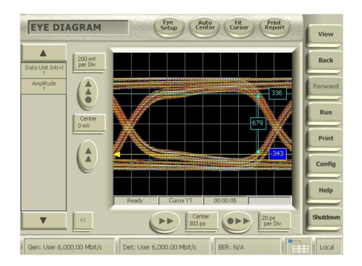
Eye Height Measured / Simulated: 679mV / 692mV
