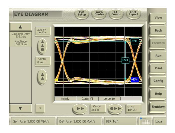
Eye Height Measured / Simulated: 890mV / 926mV
