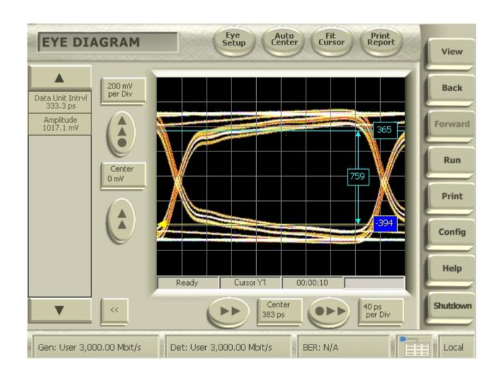
Eye Height Measured / Simulated: 759mV / 794mV
