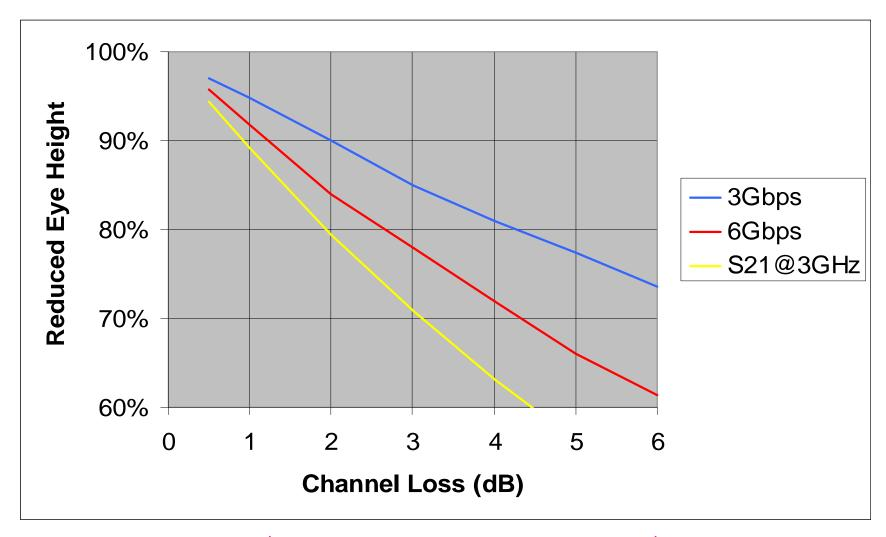
(Insertion Loss Measured at 3GHz)
