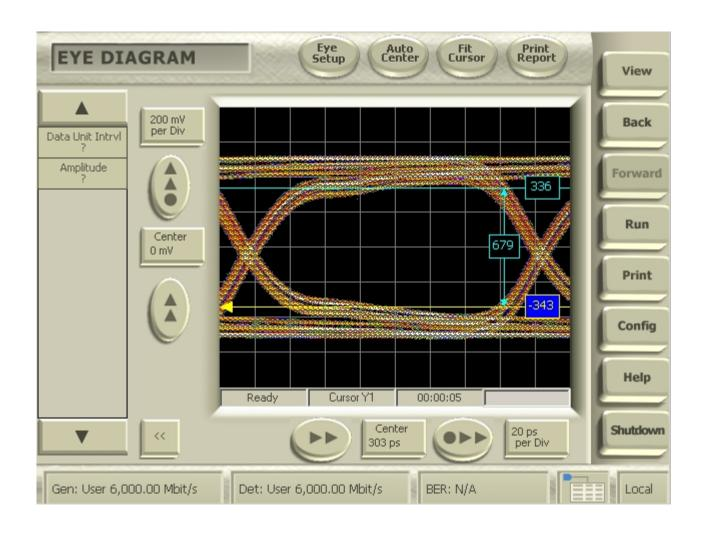
Eye Height Measured / Simulated: 679mV / 692mV
