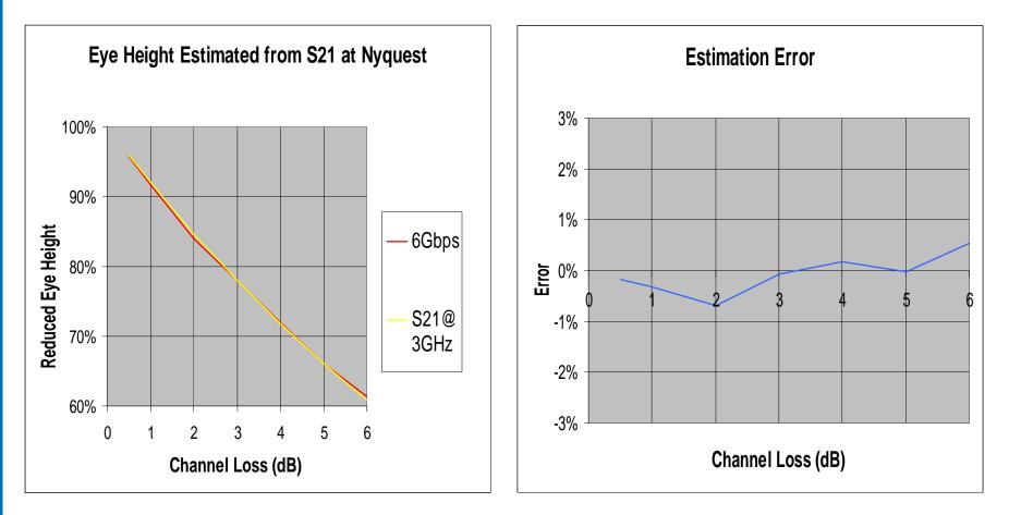
(Insertion Loss Measured at 3GHz)
