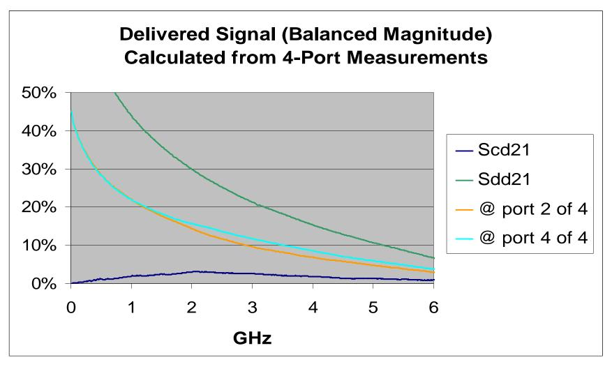
$S_{2 from _ port1 and 3} = 0.5 * (S_{21} - S_{23})$   $S_{4 from _ ports1 & 3} = 0.5 * (S_{43} - S_{41})$
