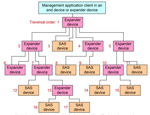
Note: Assume that the phy with the lowest phy identifier in each expander device is on the top right, and the remaining phys have increasing phy identifiers assigned in a counter-clockwise direction
