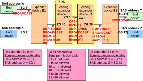
They could have zone permission tables and phy zone information and work from the SZG in the ZONED BROADCAST request, or the ZPSDS ingress boundary expander could translate between a source SAS addresses and their SZG, and the ZPSDS egress boundary expander could translate between the SZGs and the destination SAS addresses.
