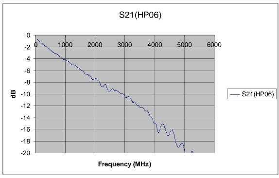
T10/05-384r2 SAS-2 Channel Models (3-Connector, Board-to-Board) HP07\_BtoB\_3Connector:
